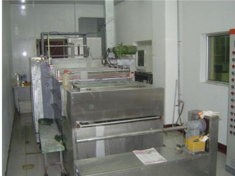
Figure 68: Film etching device at China Institute of Atomic Energy
