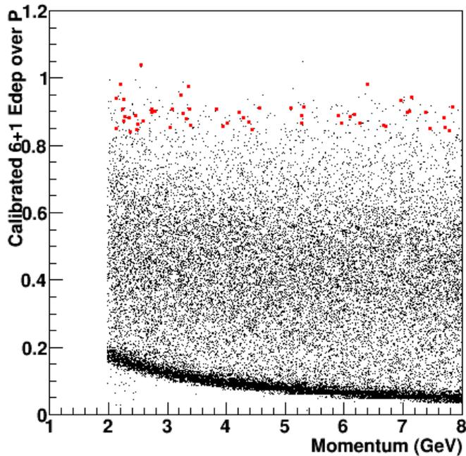
Electron Efficiency for ECAL (PS+SH) using 6+1 Clusters
