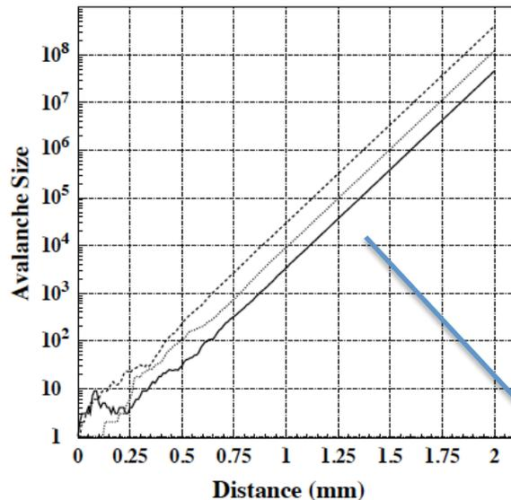
Fig. 6. Avalanches started by a single electron at  $x = 0$  for  $\alpha = 13/\text{mm}$ ,  $\eta = 3.5/\text{mm}$ . We see that the very beginning of the avalanche decides on the final avalanche size. Once the number of electrons is sufficiently large the avalanche grows like  $e^{(\alpha-\eta)x}$ .
