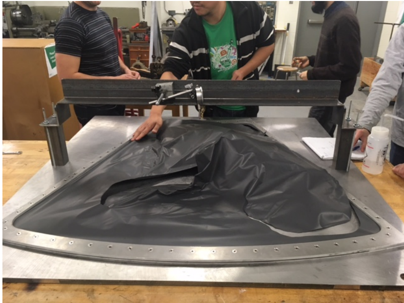
Figure 4: Photo showing the window after it burst.
