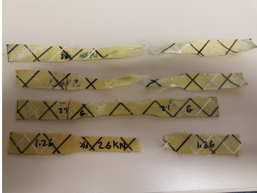
Figure 7: Stress test samples after testing. From top to bottom: Single layer, double layer, Gorilla Glue, epoxy.
