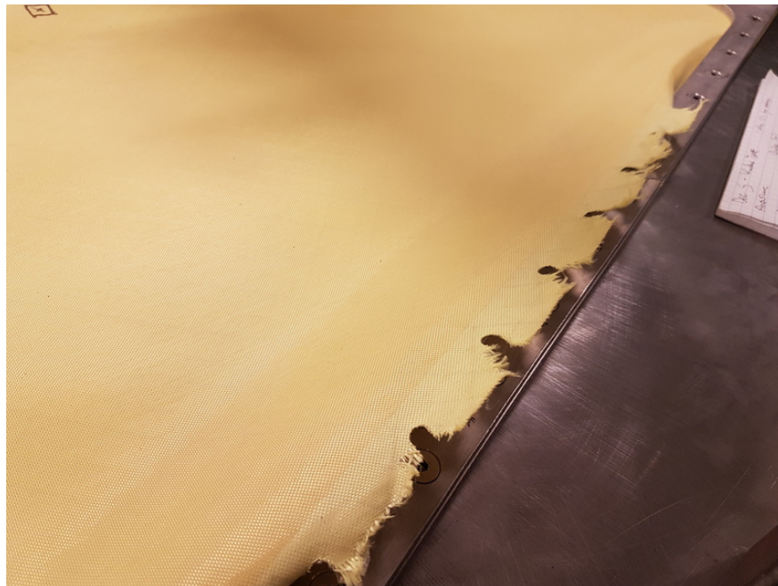
Figure 4: Photo showing the window after it failed.
