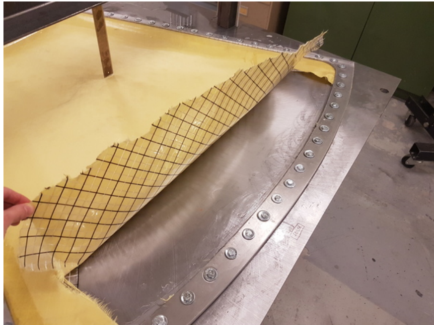
Figure 4: Photo showing the window after it failed.
