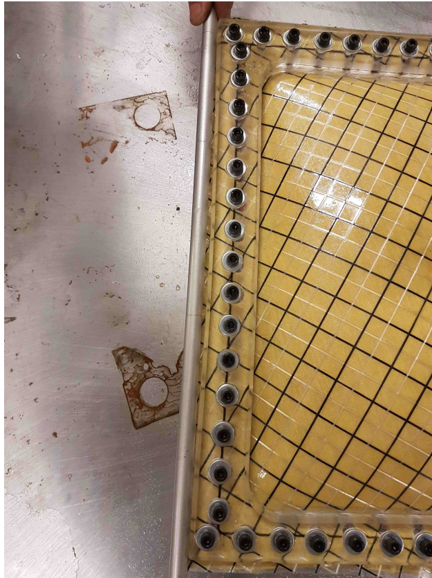
Figure 4: Inward deformation at the side of the window at 50 psi. A straight steel rod provides a reference.
