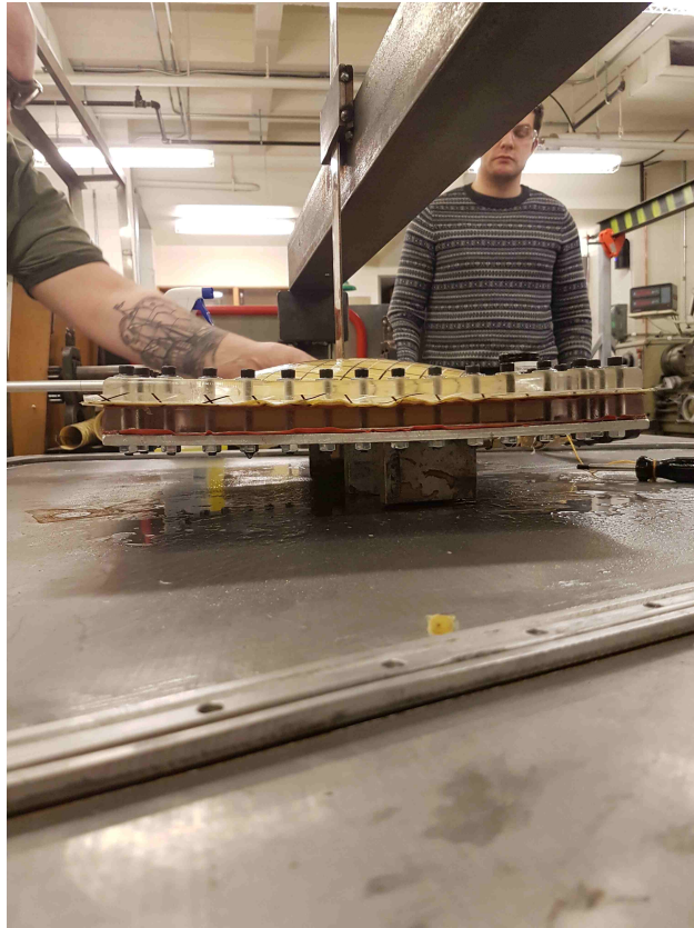
Figure 3: Side view of the window frame and plate, showing the upward deformation at 50 psi.
