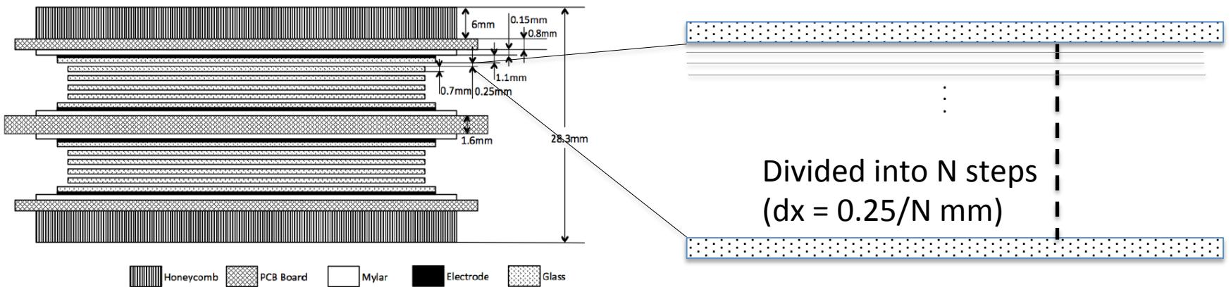
Figure 108: The structure of the MRPC prototype
