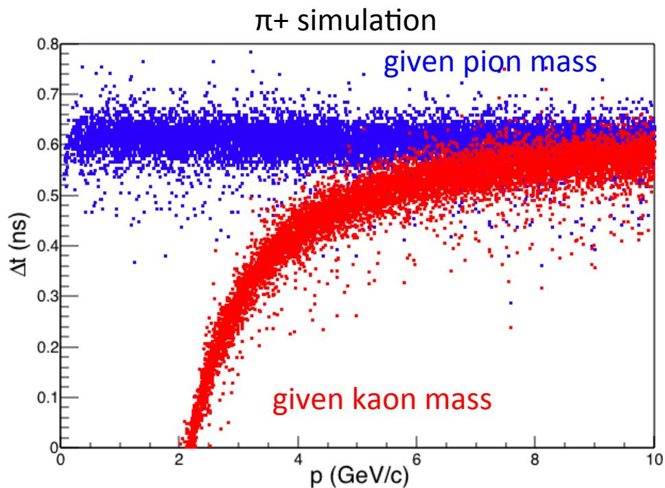
$$\Delta t = \text{time\_measured} (t_{\text{Ref}} + t_{\text{Leading}}) - \text{time\_expected}$$
