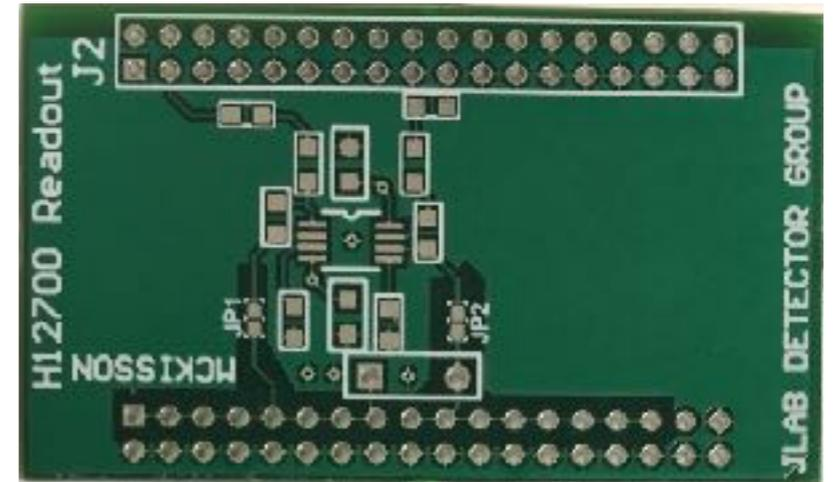
Blade board prototype (with 3 different sum configuration: sum of 2, 4, 8 channels)
