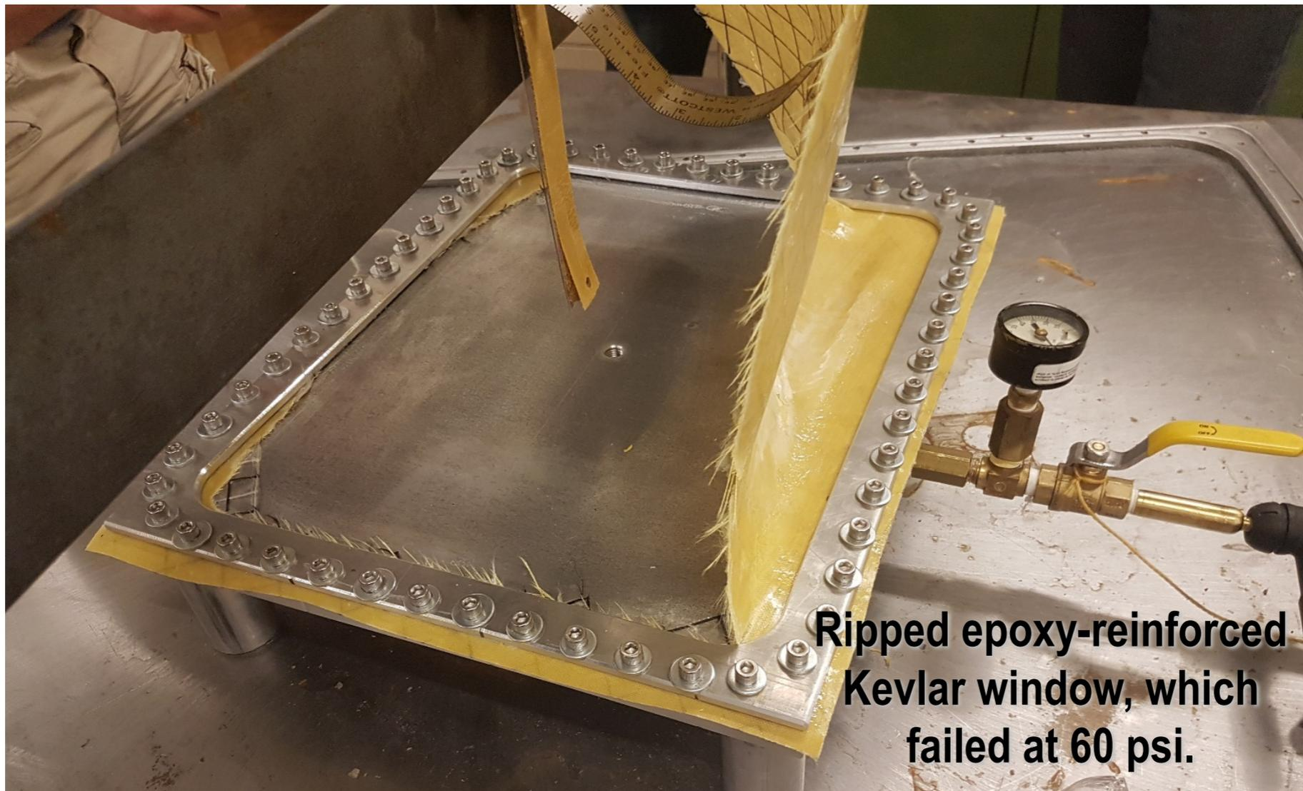
Ripped epoxy-reinforced Kevlar window, which failed at 60 psi.
