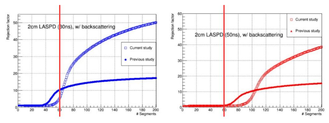
Looks like x60 azimuthal segmentation is no longer good enough. We need 120 segmentations. - challenges: higher cost; smaller side for readout (lower light yield?); very tight room if doubling need of light guides and FMPMTs.
