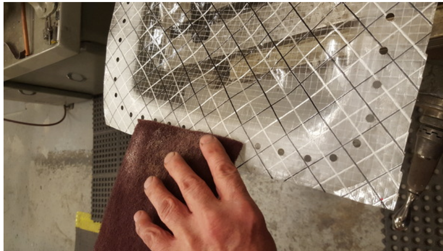
Figure 7: Sanding the mylar layer for better bonding with epoxy mixture.
