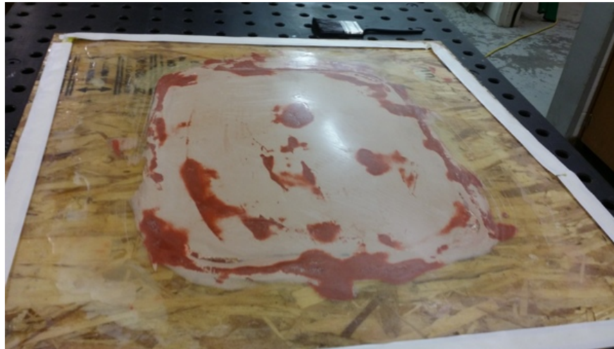
Figure 1: Pre-formed shape of the window-shell (Note: The shape of this mold was modeled after the small window-shell shape at \sim 10 psi pressure.)
