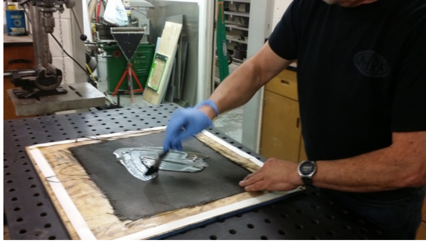
Figure 2: Applying epoxy to carbon layer. (Note that this was done without vacuum bagging.)
