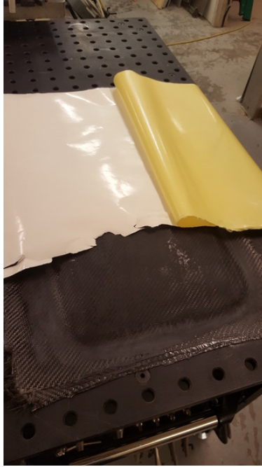
Figure 3: Cured window shell and Kevlar before applying the final layer.
