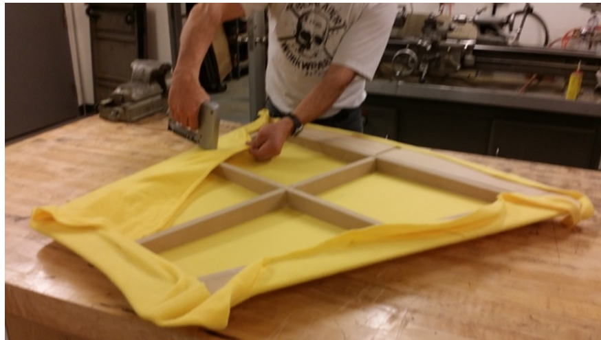
Figure 11: Tightening the foam cloth on the wooden frame.
