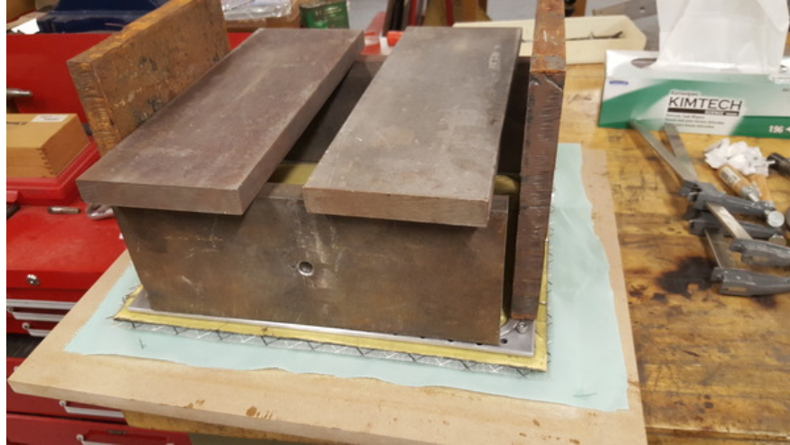
Figure 9: Metal blocks used as weight after applying epoxy mixture.
