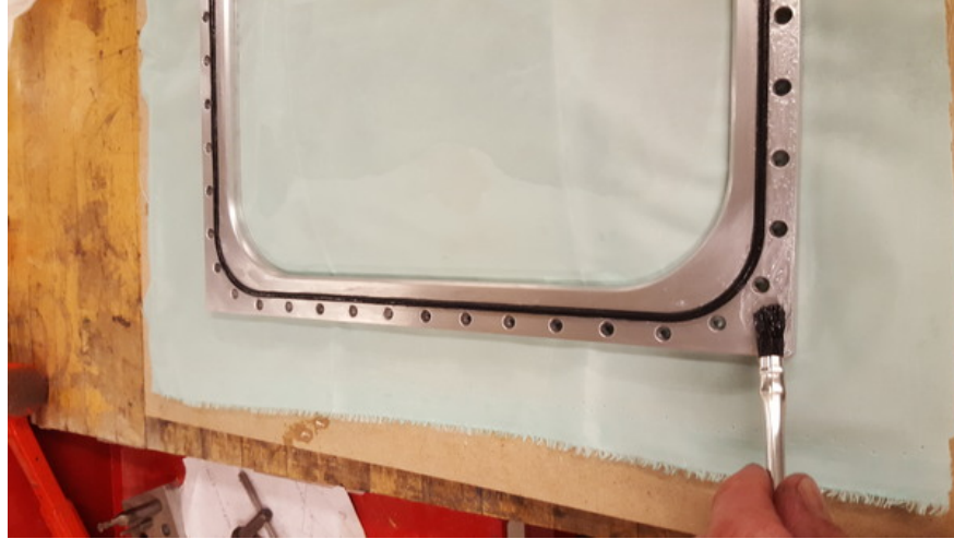
Figure 6: Applying epoxy mixture on the metal frame.
