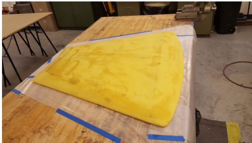
Figure 12: The end product after applying a thin epoxy mixture layer left to cure overnight.
