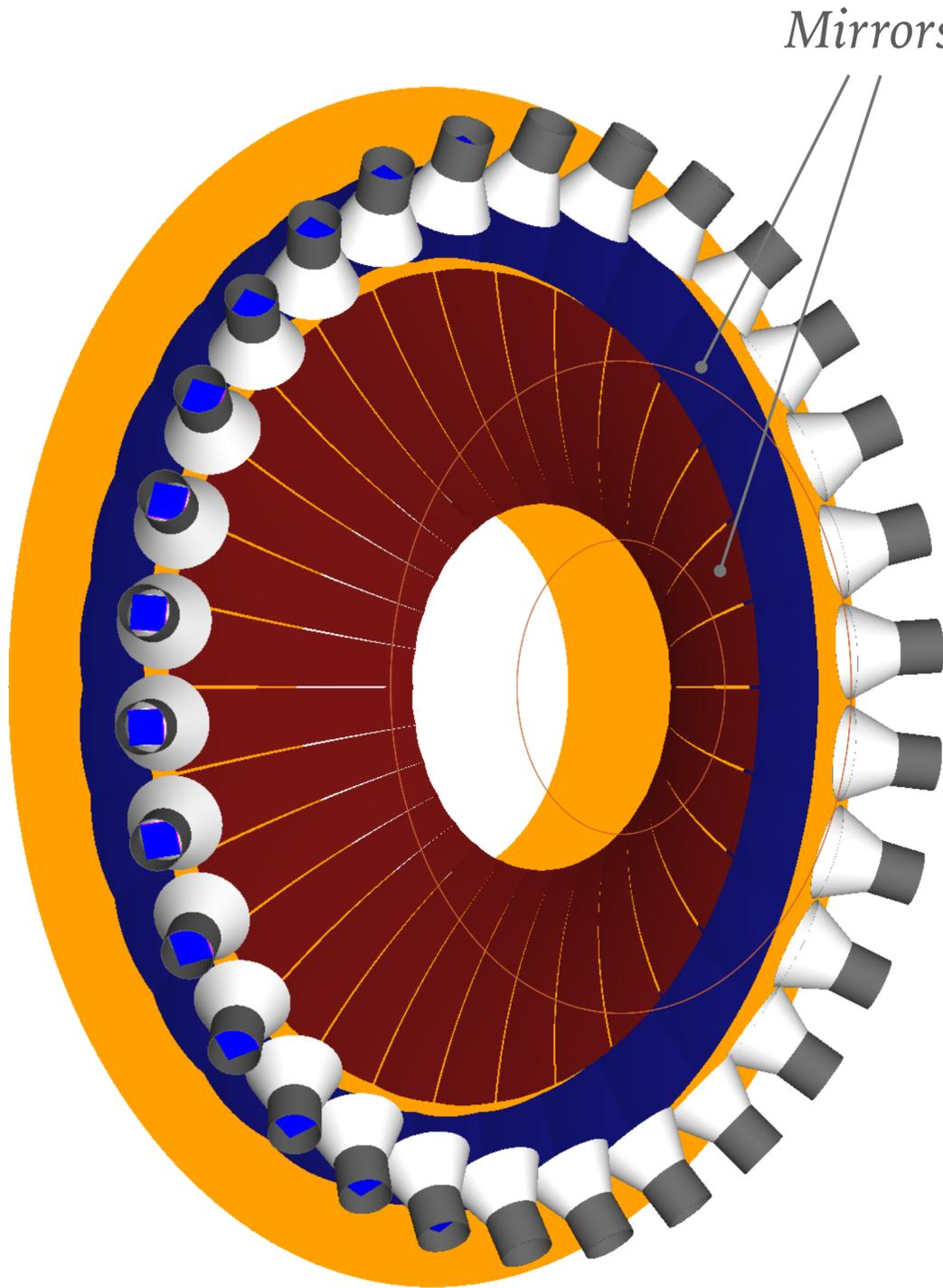
➤ Each sector consists of an inner and outer mirror. In the PVDIS configuration, both mirrors are in acceptance, where only the inner mirror is used for J/Psi & SIDIS.
