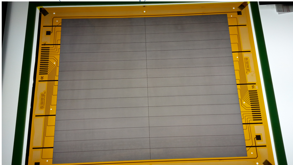
Flexible 2D readout board (CERN PCB workshop)
