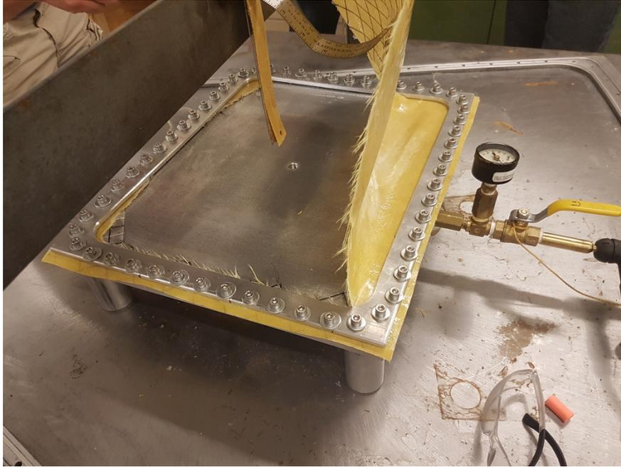
Figure 5.23: Mylar-Kevlar window after bursting during Test 4.
