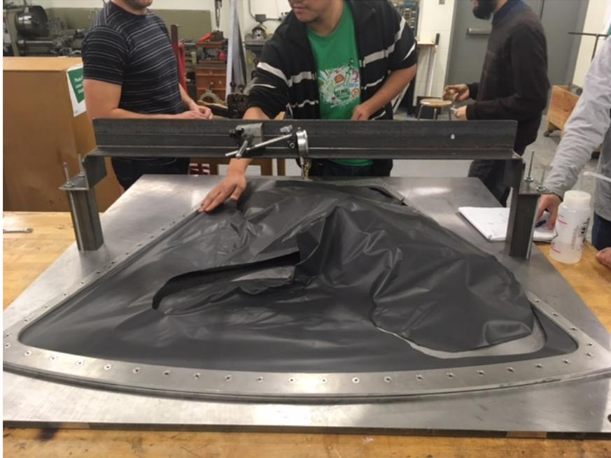
Figure 5.13: Aftermath of failure of the PET/Tedlar window.
