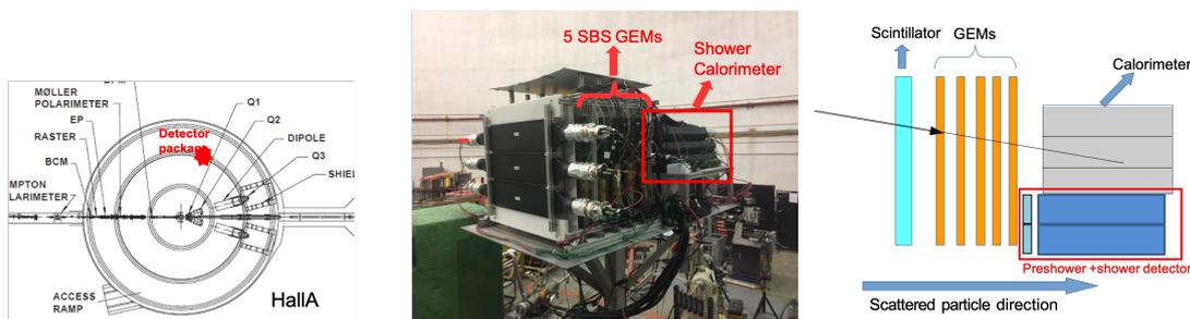
Figure 10-10: Left: Top schematic view of Hall A and the location of the test equipment. Middle: The picture of detector package. Right: illustration of the detector setup. Three shashlik prototypes are stacked together, with preshowers are placed in front.
