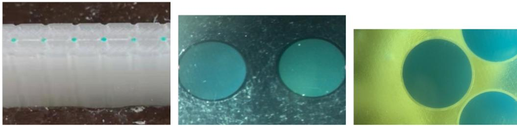
a) Fiber and fiber end reflector    b) WLS fiber and clear fiber    c) Fiber and PMT window
