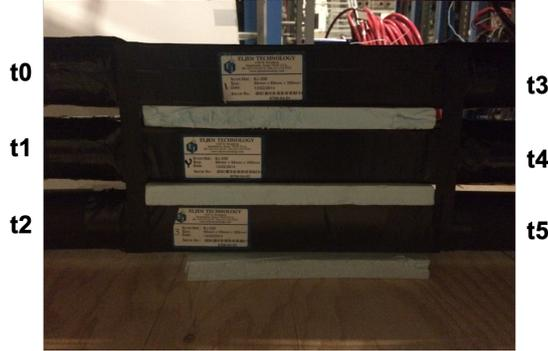
Figure 1-1: The picture of 3-bar test setup. Each scintillator bar is read out by both sides, and the time  $t$  means the time of each PMT. A blue foam is placed between scintillators to make sure the gap distance is same.
