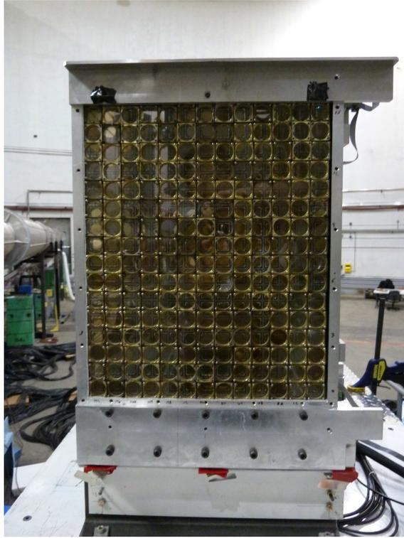
Figure 3-8: The front view of DVCS calorimeter. The  $PbF_2$  blocks are revealed with removed front plate.
