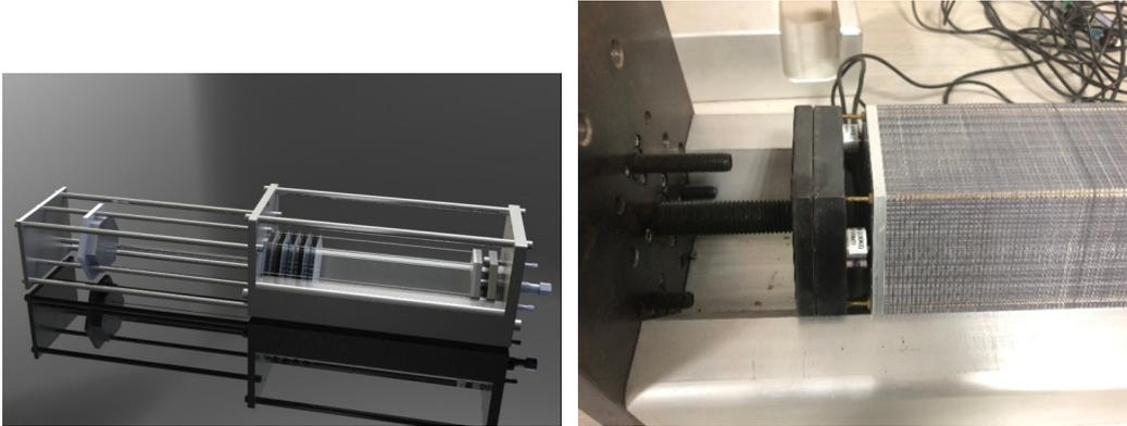
Figure 9-8: Left: Assembly tool for shashlik shower module. Right: The module in compression. Three pressure sensors are placed between the steel plated and shashlik detector to monitor the pressure.
