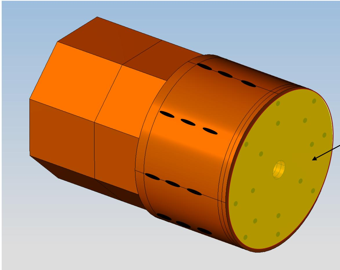
With new endcap motion concept the rear backplates are no longer available to route cables out of endcap
