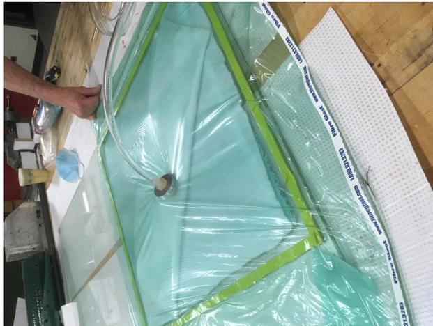
Figure 19: The vacuum being pulled on the small Carbon fiber window.
