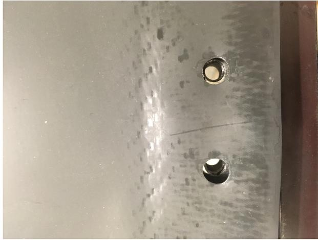
Figure 31: The Tedlar scratched by the leaks.
