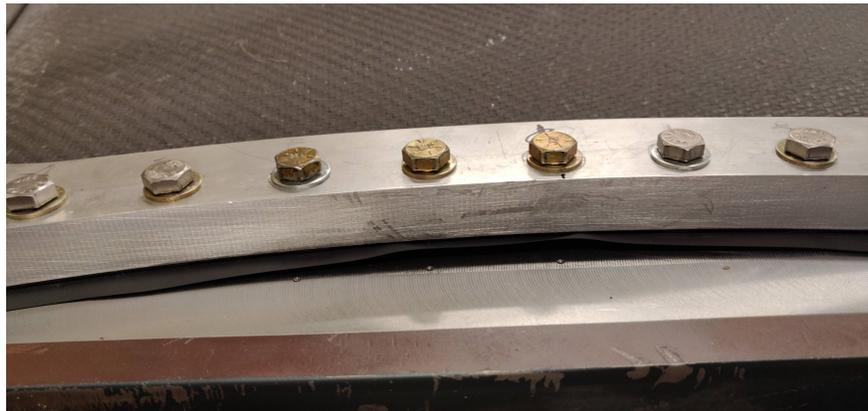
Figure 30: The Tedlar peaked out of the frame while being inflated.
