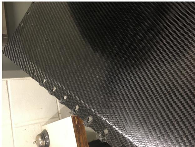
Figure 36: Torn and stretched bolt holes on the carbon fiber window.
