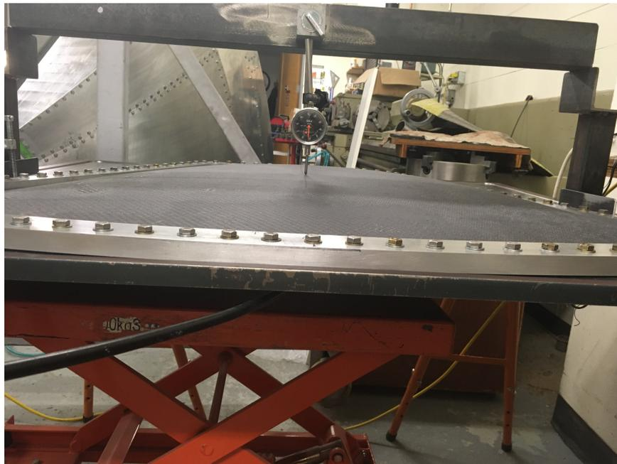
Figure 34: The carbon fiber window bulging more on the right side.
