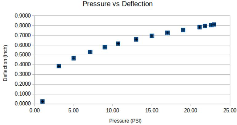
Figure 9: Test 2.1 A graph showing the relationship between pressure and deflection for the second test in imperial units.
