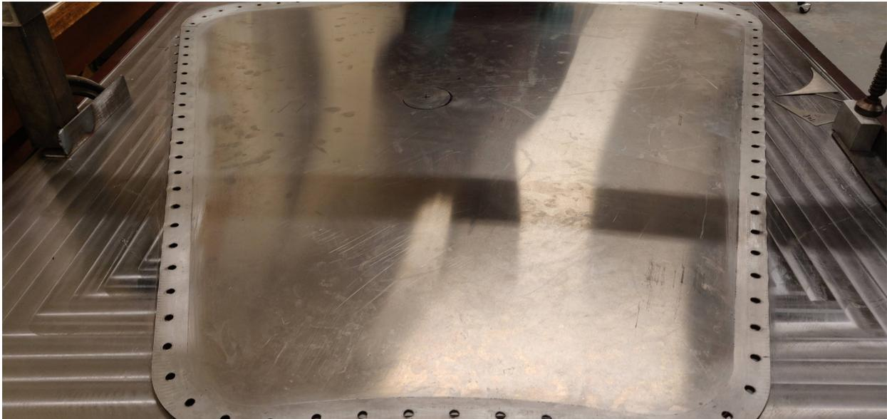
Figure 13: The aluminum window's bolt holes on February 18th. Stretching is observed around some bolt holes on the left.
