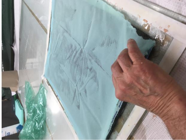
Figure 18: The nylon is placed over the breather and bleeder cloth.
