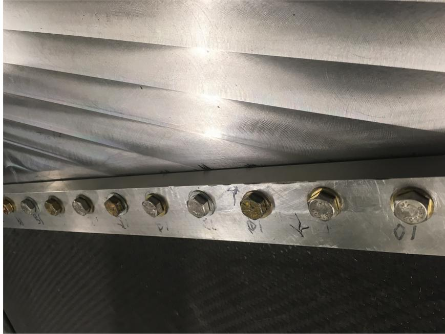
Figure 35: Stress on the window forcing out some shards of the carbon fiber window beyond the frame.
