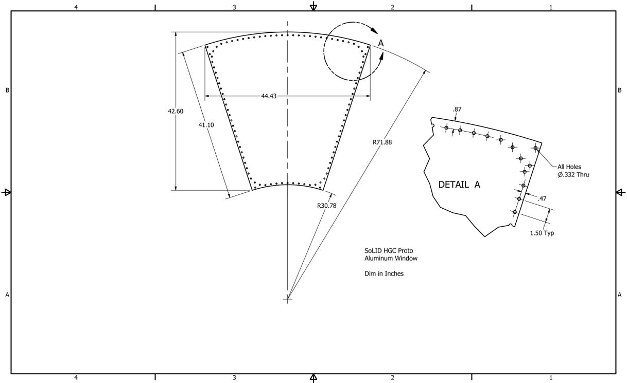
Figure 1: A technical drawing of the front window drawn by Gary Swift. All dimensions are in inches.
