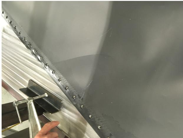
Figure 32: Creases in the Tedlar were also found near leaks.
