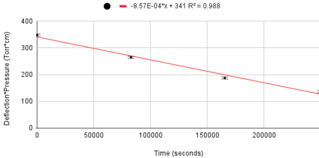
Figure 29: The deflection and pressure from the last time the window was pumped to 26 psi. This rate was used to calculate the leak rate of the carbon fiber window.
