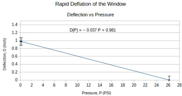
Figure 12: Test 3. The window's rapid deflation.
