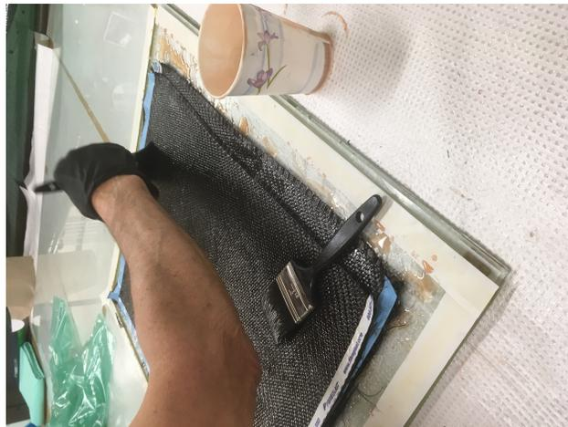
Figure 17: The epoxy was brushed in a dabbing motion to pull the epoxy through the carbon fiber with no air bubbles.
