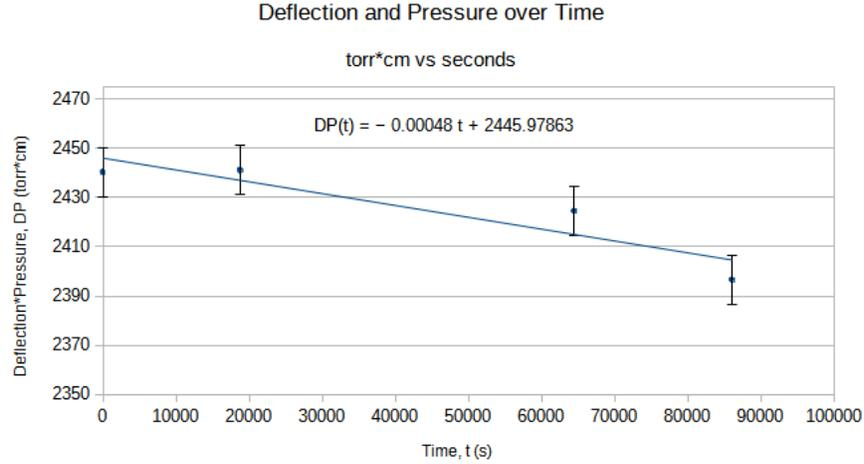
Figure 10: Test 2.2 The deflation of the aluminum window over time.
