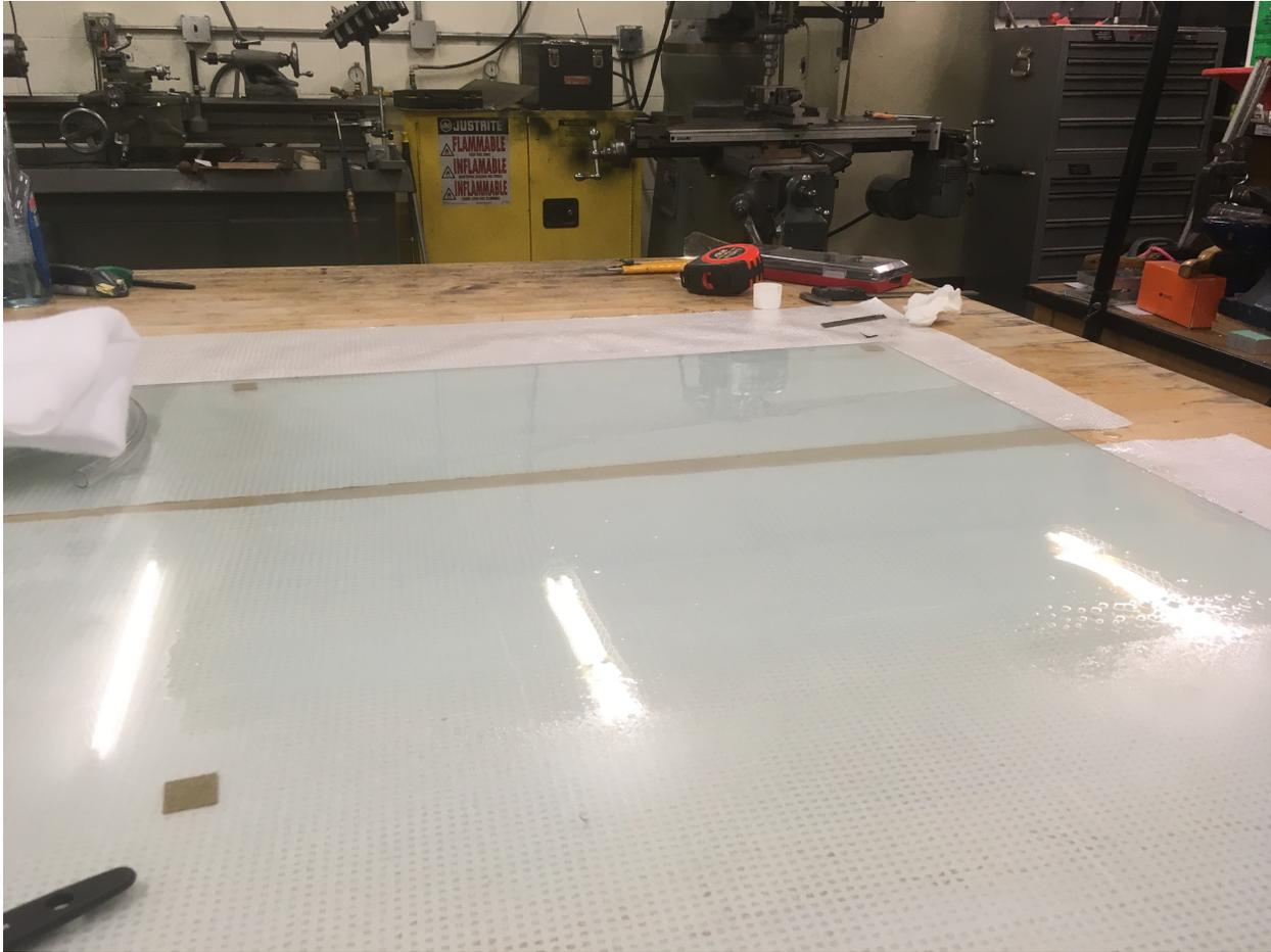
Figure 16: “Fisheyes” that formed when the release agent dried.
