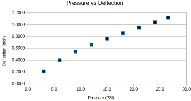
Figure 8: A graph showing the relationship between pressure and deflection for the first test in imperial units.
