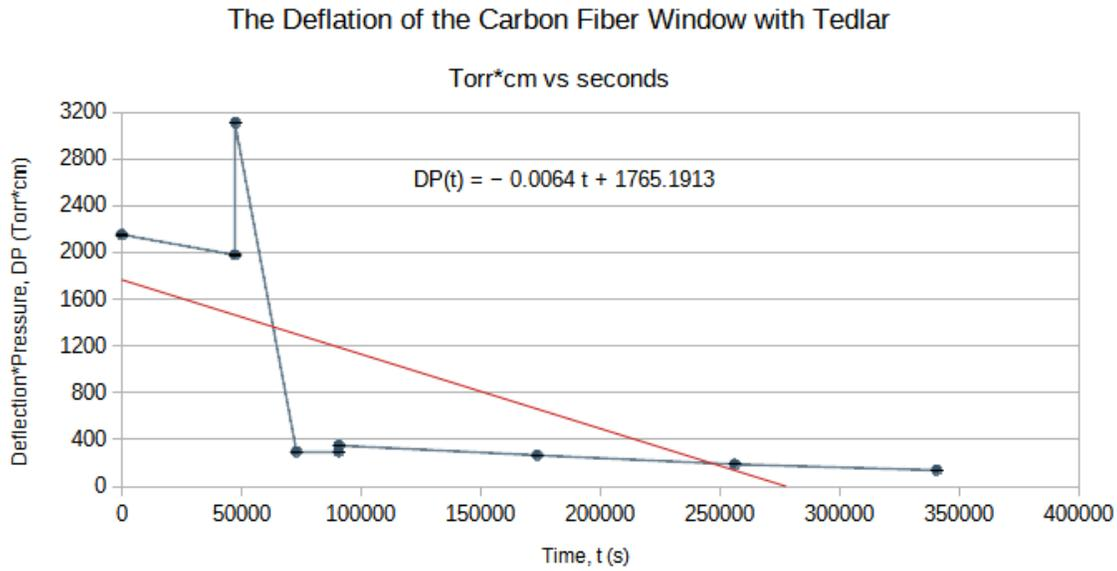
Figure 28: The deflection and pressure over time. It is clear from this graph that the window had a leak.
