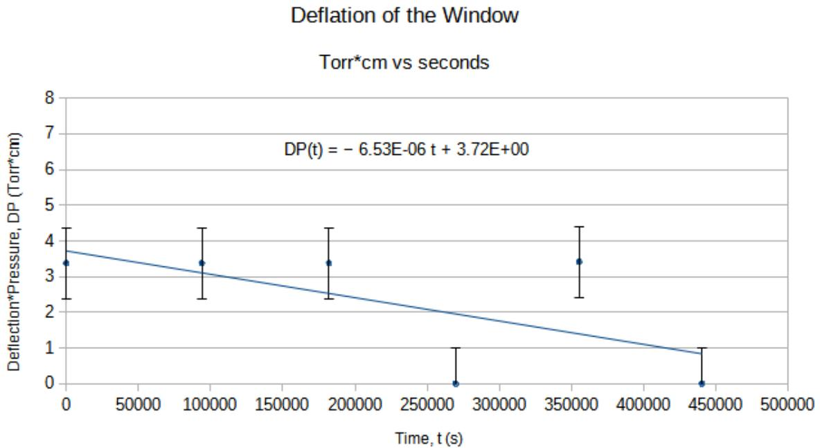
Figure 11: Test 2.4 The rate is  $(-7 \pm 4) \times 10^{-6} \frac{\text{Torr}\cdot\text{cm}}{\text{s}}$ .
