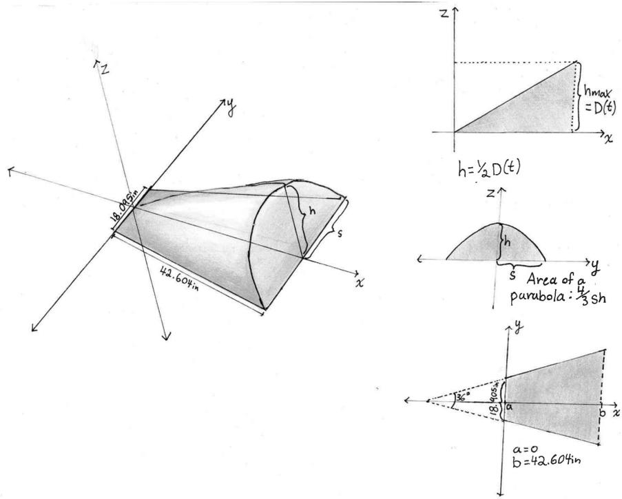
Figure 7: Model of the volume of the window. The height  $h$  varies over time. The maximum value for  $h$  is the deflection of the window at its highest point
