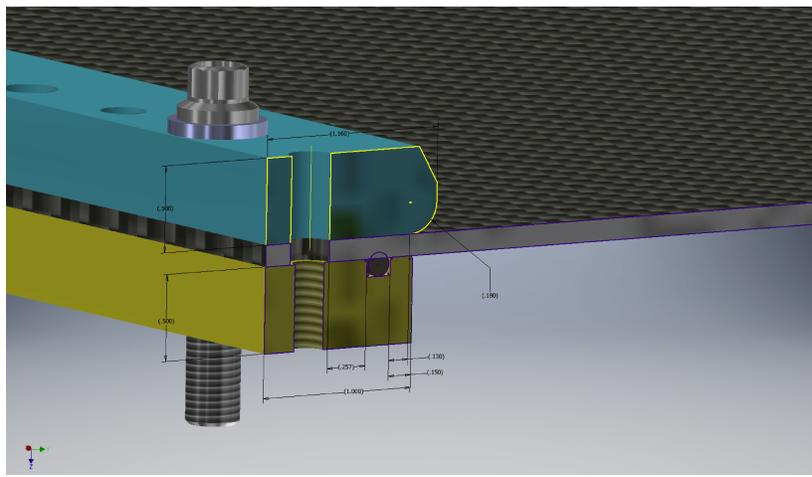
Figure 2: A 3D rendering of the window frame and the O-ring groove
