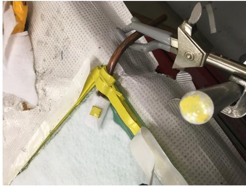
Figure 25: This vacuum setup prevents the window from becoming distorted.
