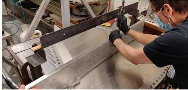
Figure 5: A level ring is used to find the highest point of the window deflection.
