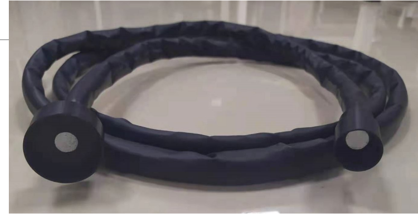
Chunhui fiber bundle connector one piece for one Ecal tower 3m PMMA clear fiber bundle
