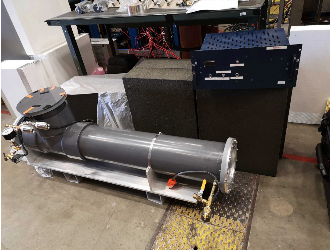
The “smaller” LGC prototype (2x2 tile of MaPMTs)
