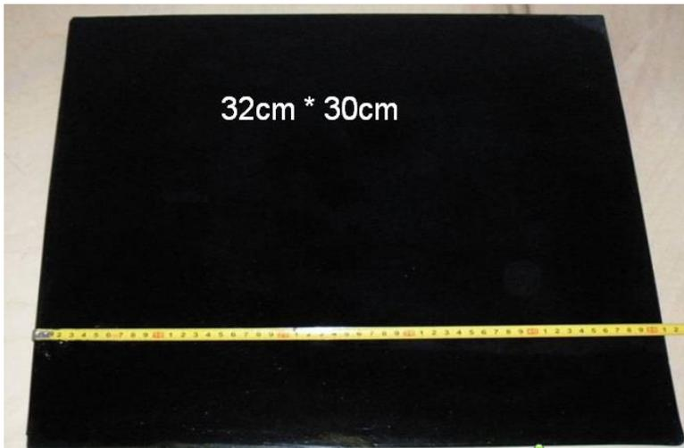
With the low-resistive glass developed in Tsinghua, resistivity has decreased by 2 orders of magnitude. (common float glass:  $10^{12} \Omega\text{cm}$ , low-resistive:  $10^{10} \Omega\text{cm}$ )
