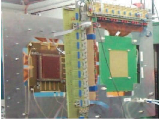
Figure 6: GEM chambers of the prototype tracker being prepared for the beam tests during hall A PREX experiment.
