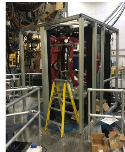
Frame to hold iron magnet shielding installed
