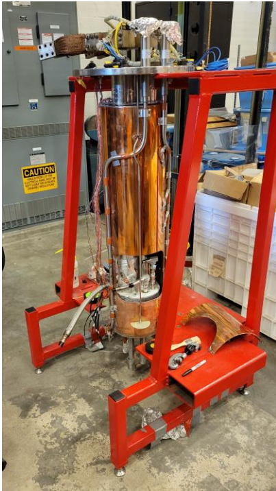
Service turret cleaning and N2 circuit mods
