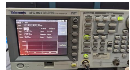
LED DC mode: generator in burst mode to mimic DC power, only key parameter is low amplitude, typical at 2.056v or 2.085v
