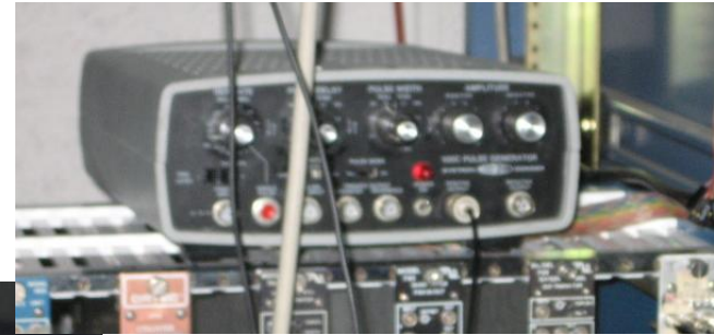
Pulser which controls the green LED
