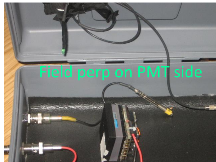
Magnetic field probe in position for field measurement
