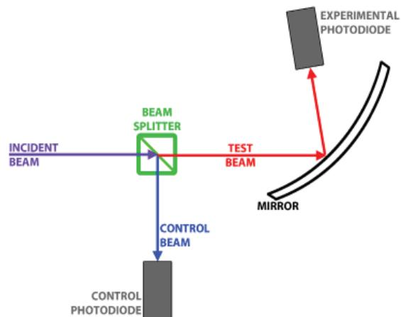
FIG. 5. System diagram for reflectivity test station.
