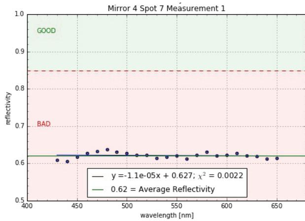
FIG. 7. Reflectivity at a visually identified smudged/scratched area.
