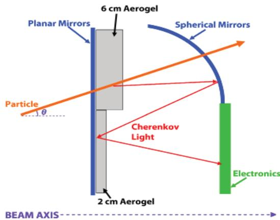
FIG. 1. Schematic of the RICH detector.
