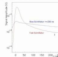
Slow Scintillator BC-444 ( $\tau \sim 250 \text{ ns}$ ) in the first 5.2  $X_0$ . Signal sampled with 2 different gates (NARROW = 55 ns, WIDE = 600 ns). Light Yields Ratio  $\frac{Q_{WIDE}}{Q_{SLOW}} \sim 2$  to be optimized.
