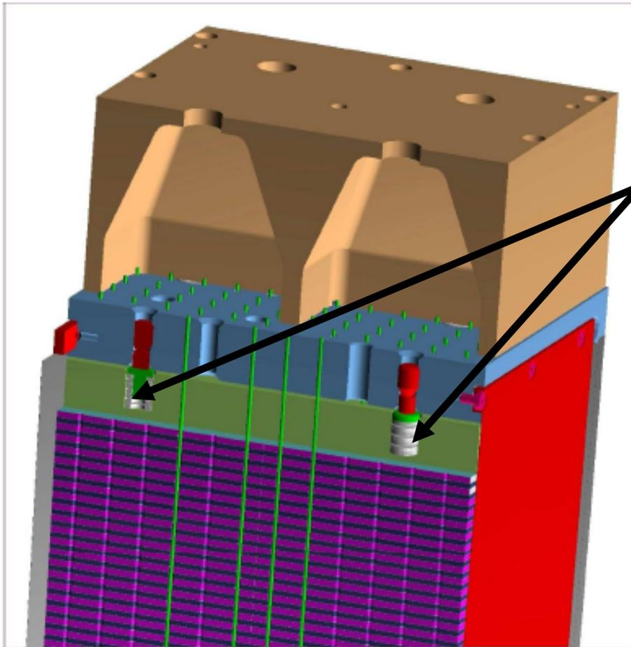
**Module Mechanical Design incorporates non-linear springs for stability against thermal excursions**
