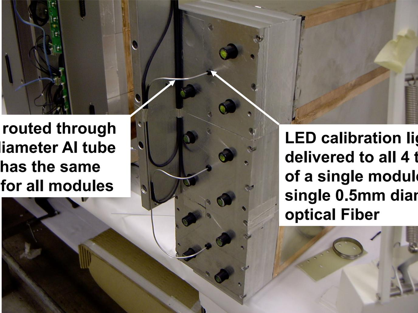
Fibers routed through 1mm diameter Al tube which has the same shape for all modules
