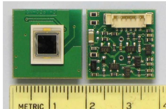
**Figure 4.32:** The Avalanche PhotoDiode (left) mounted on the back of the Charge Sensitive Preamplifier (right) used by PHOS and EMCal.
