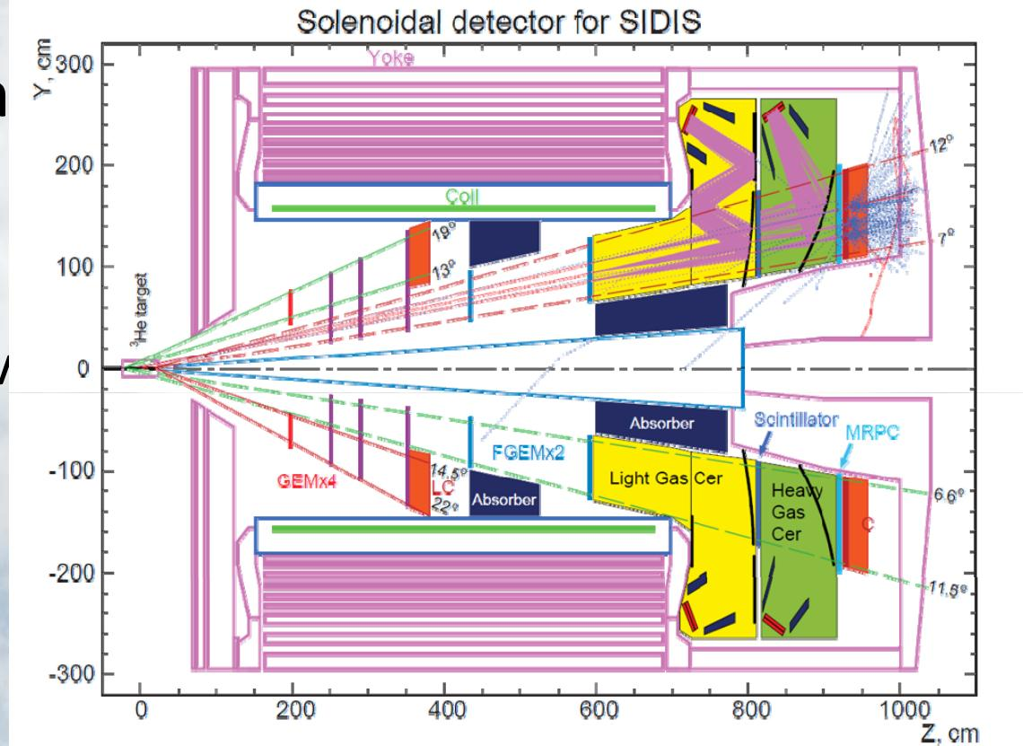
Additional devices of MRPC, scintillator plane, heavy gas Cerenkov which provide us the capability in hadron detection.
