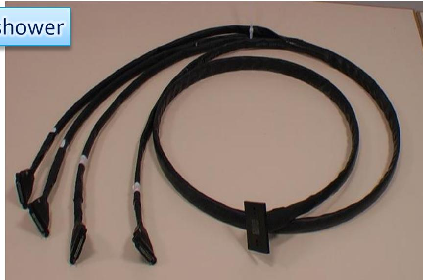
• fiber bundle to PMT connector, cost estimate \$25/module
