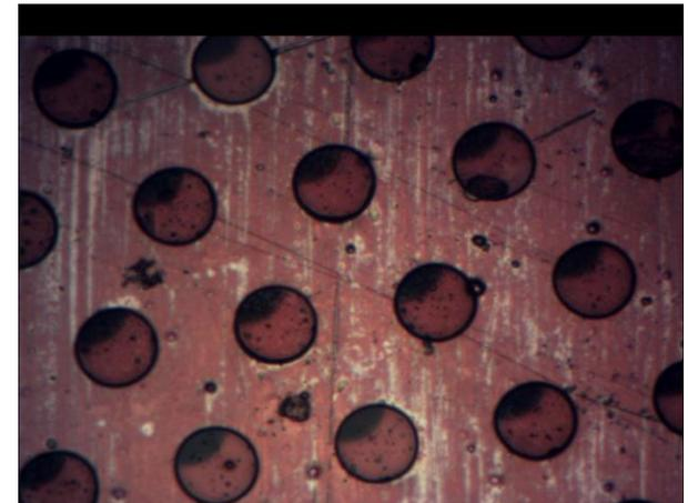
A GEM foil produced with top and bottom mask misaligned
