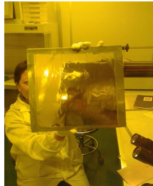
A 30*30cm 2 GEM foil produced at CIAE
