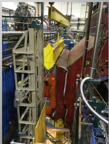
Outer two layers of NORTH and UP-NORTH sectors of CLEO removed.
