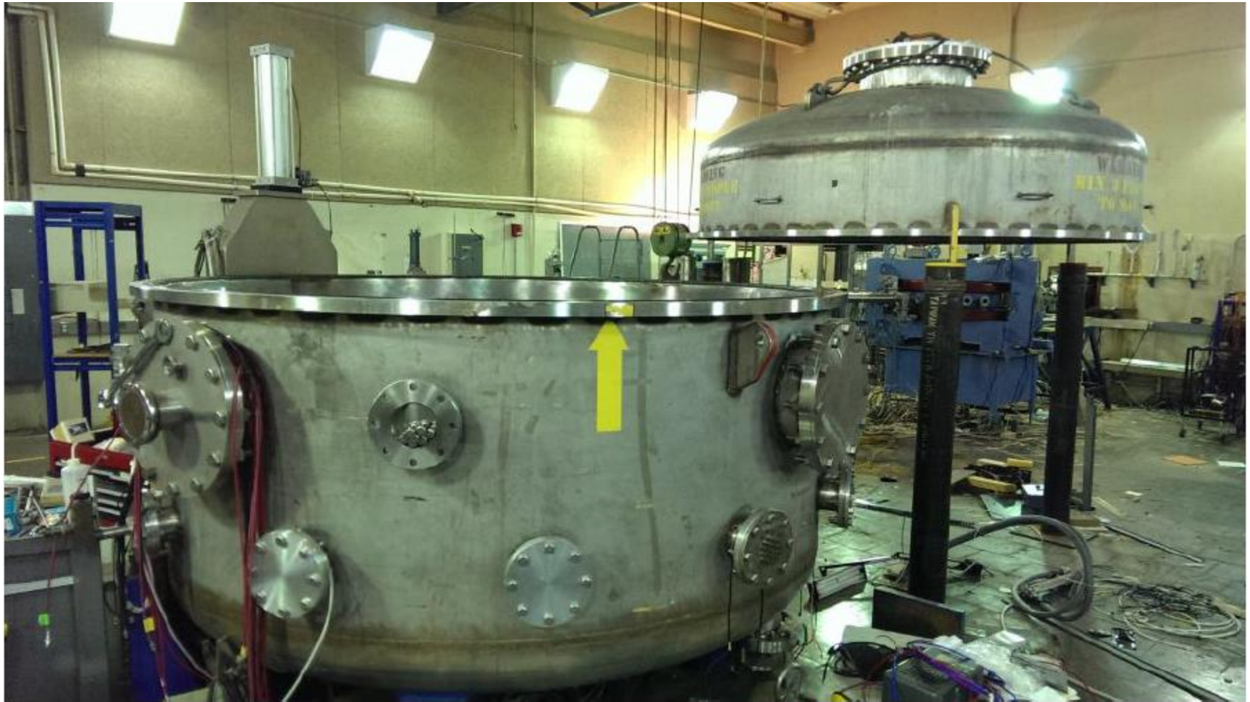
Figure 37 Large size evaporator "Big Mac" at SBU.
