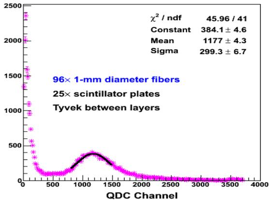
1.5 mm Scintillator Plates, XP2262, HV = -2100 V
