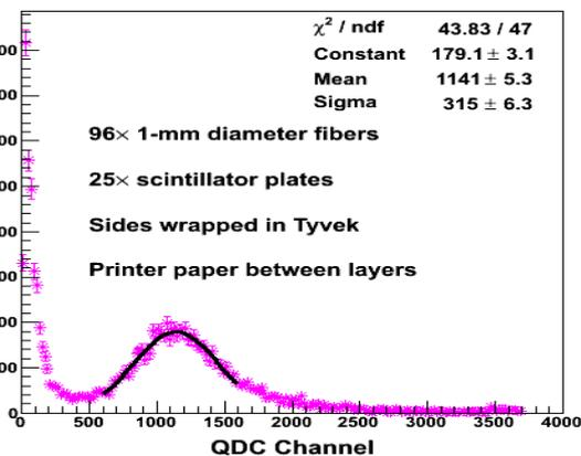
1.5 mm Scintillator Plates, XP2262, HV = -2100 V
