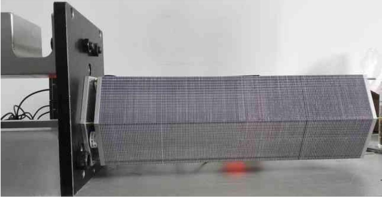
SDU now have two modules (no fiber), one 170-layer with inner sensor for mechanic testing; one full module
