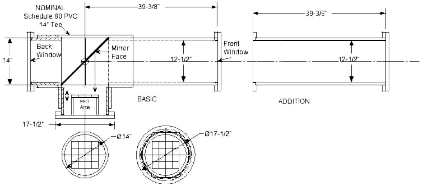
Figure 8: Tank design for the telescopic Cherenkov device.
