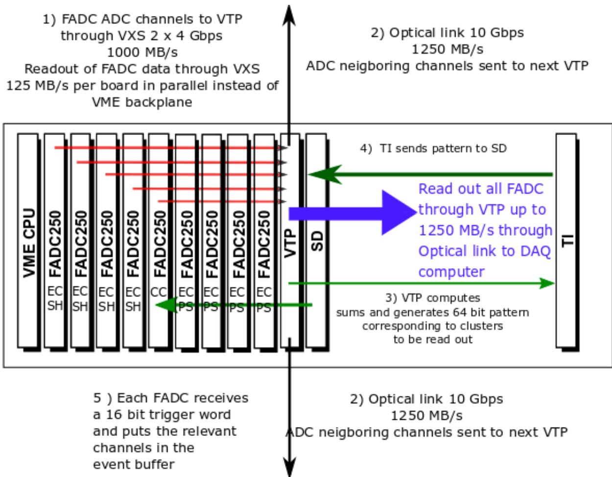
Figure 3: VXS crate module configuration for PVDIS
