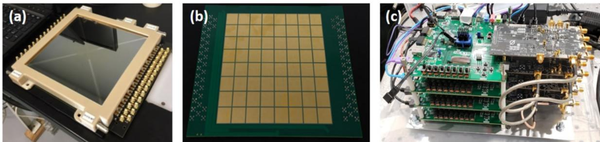
Figure 10: a) The 20x20 cm<sup>2</sup> LAPPD device, and (b) 8x8 array, 25x25mm<sup>2</sup>, 64-pixel readout. (c) The Nalu ASoC data acquisition system, each evaluation board has 4 readout and attached to one FPGA, evaluation boards can be stack together for multi-pixel readout.
