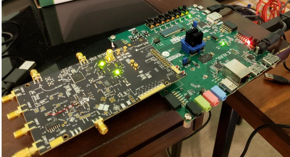
Figure 7: NALU ASOC evaluation board on a NEXSYS FPGA evaluation board
