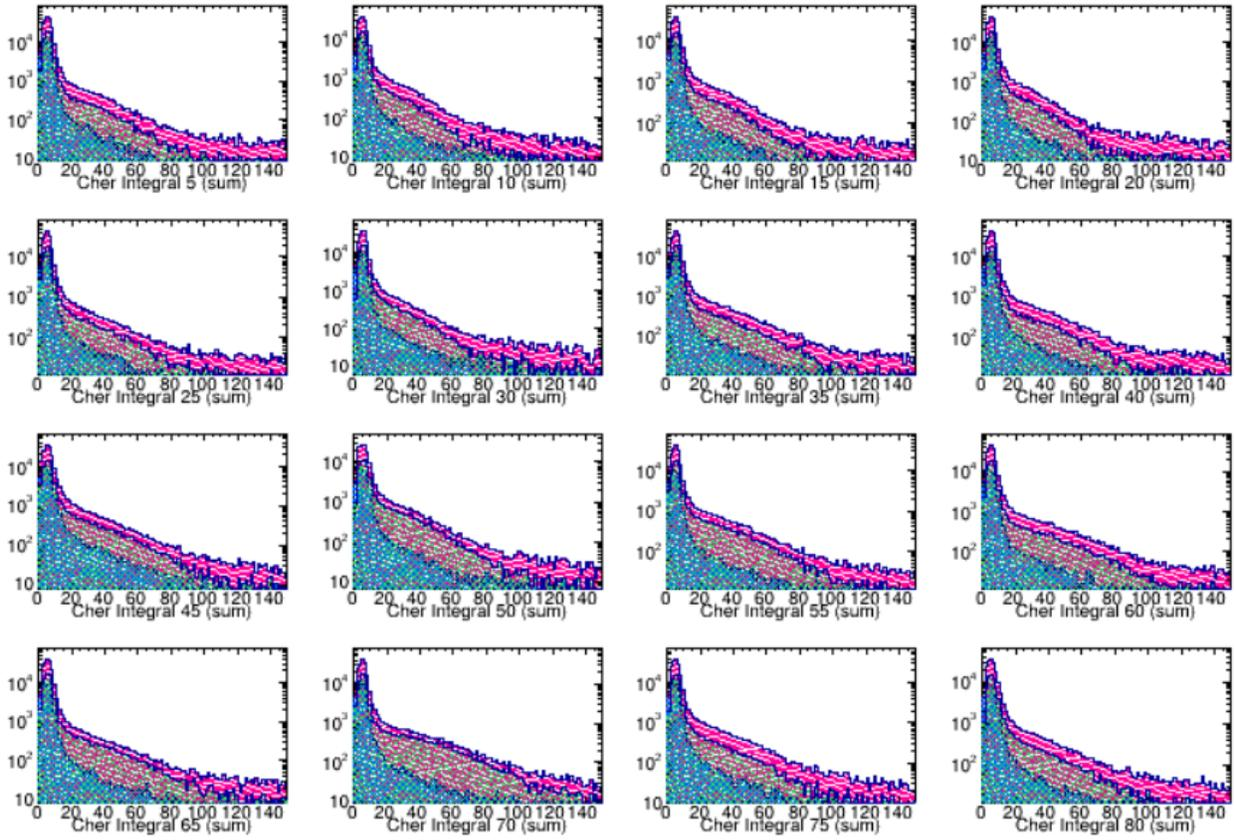
Figure 19: Beam data: charge integral in pC (FADC250s in mode 3) from all 16 MaPMTs (sums signal only, plots of quad signals are also available but not shown). Different histograms are obtained with different timing cuts as explained in the text.
