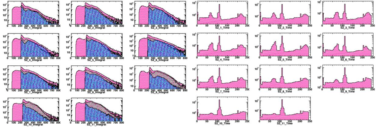
Figure 17: Beam data (FADC250s in mode 3) from the second scintillator plane. The charge integral in pC (left) and the timing distributions in ns (right) are shown. The two different distributions in the charge integral plot are obtained with different timing cuts.
