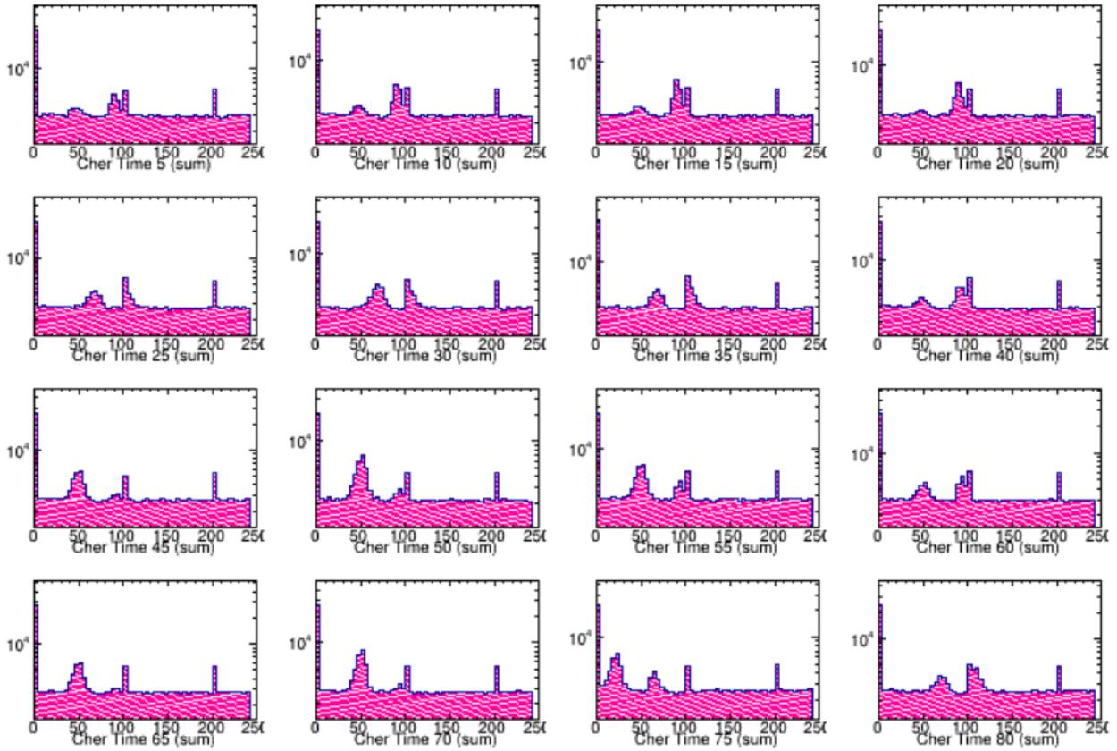
Figure 20: Beam data: timing distribution in ns (FADC250s in mode 3) from all 16 MaPMTs (sums signal only, plots of quad signals are also available but not shown).
