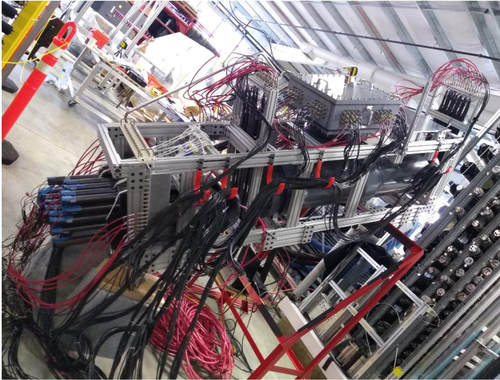
Figure 5: Picture of the Cherenkov test stand as assembled in the ESB building at Jefferson Lab.
