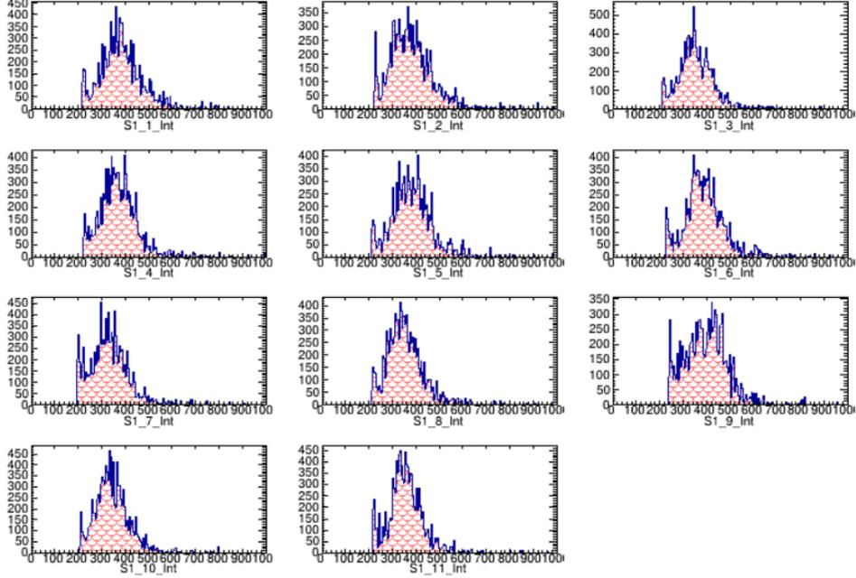
Figure 13: Plots of the integrated charge distribution per channel (in pC) in the first scintillator plane (the plane that is placed at the front of the Cherenkov tank).
