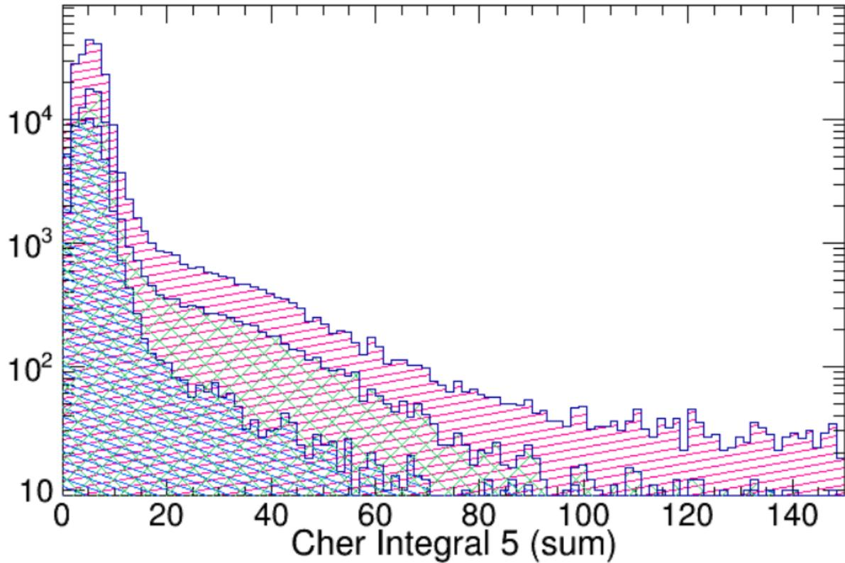
Figure 8: Beam data: charge integral in pC, FADC250s in mode 3. Here only one of the 16 MaPMTs is shown (sums signal only, plots of quad signals are also available but not shown). The charge integrals from all the other maPMTs are shown in the Appendix. Different histograms are obtained with different timing cuts as explained in the Appendix.
