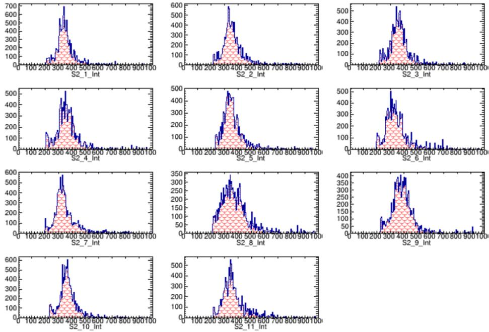
Figure 14: Plots of the integrated charge distribution per channel (in pC) in the second scintillator plane (the plane that is placed at the back of the Cherenkov tank).
