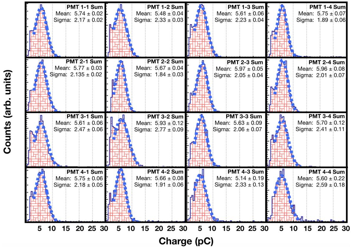
Figure 7: Plots of the integrated charge distribution per MaPMT (in pC) corresponding to one photoelectron (data taken with a random trigger).
