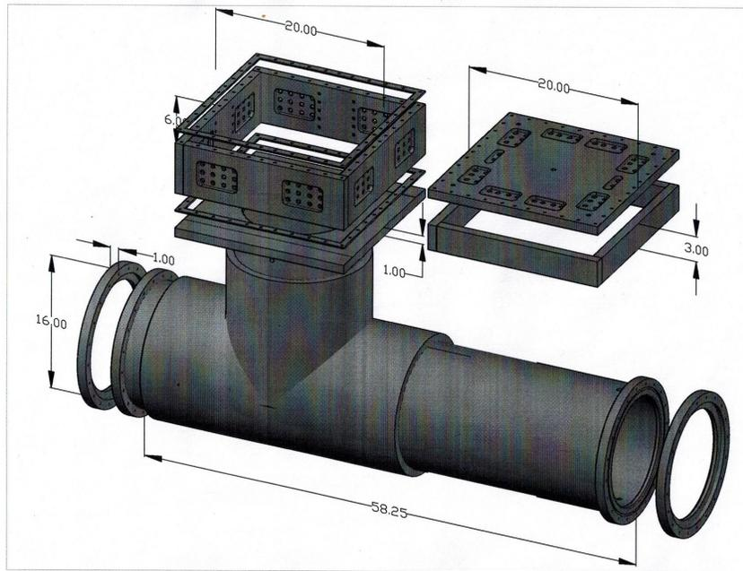
Figure 2: The Cherenkov tank design, as delivered to Jefferson Lab. The schematic shows both the electronics housing box for the MaPMT summing board and the housing for the LAPPD electronics.
