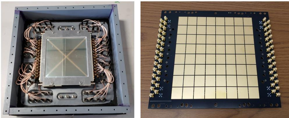
Figure 4: (left) Pixel GEN II-LAPPD coated with wavelength shifter was installed in housing ready for swapping with MaPMTs. (right) The  $8 \times 8$  array  $25 \times 25 \text{ mm}^2$  pixel readout board attached behind the LAPPD, the pixel size is exactly the same size as a quadrant of MaPMT.
