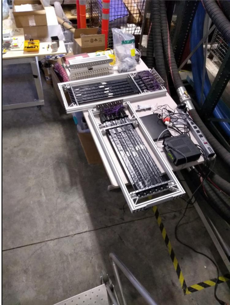
Figure 10: Picture of scintillator planes used in the detector package for the Cherenkov test. Each of the the 2 planes have 11 bars with a rough overlap between adjacent bars of about 0.25 inch. The scintillating light is collected at one end only by a 0.5 inch Hamamatsu PMTs.
