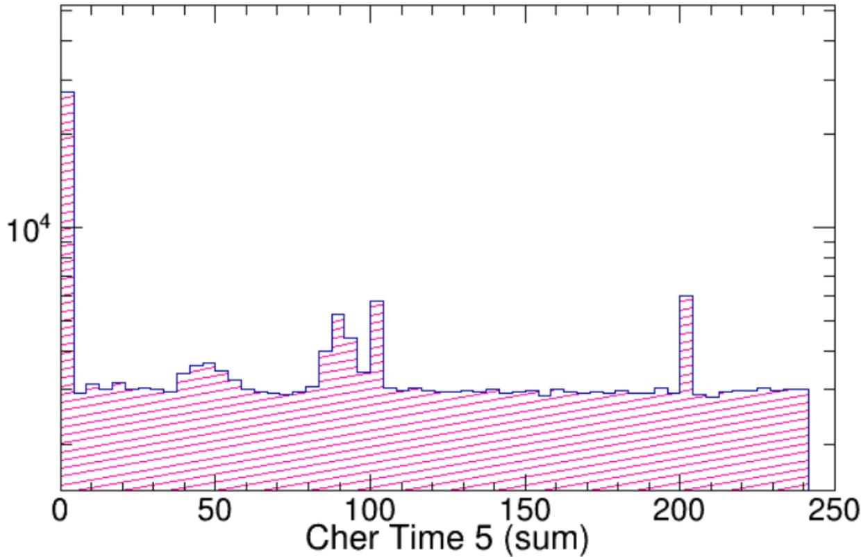
Figure 9: Beam data: timing distribution in ns, FADC250s in mode 3. Here only one of the 16 MaPMTs is shown (sums signal only, plots of quad signals are also available but not shown). The timing distributions from all the other maPMTs are shown in the Appendix.
