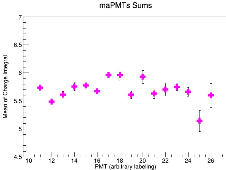
Figure 15: Mean from a Gaussian fit to the integrated charge distribution per maPMT (in pC) corresponding to one photoelectron (data taken with a random trigger).
