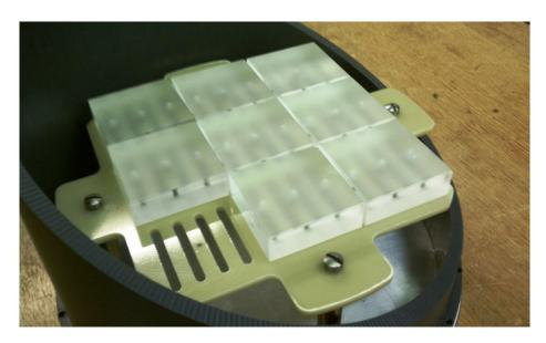
Figure 72: PMT assembly mounting prototype showing  $3 \times 3$  array of dummy PMTs inside the space restricted by magnetic shielding.
