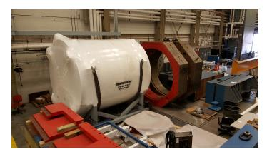
Figure 6: CLEO II magnet at JLab.
