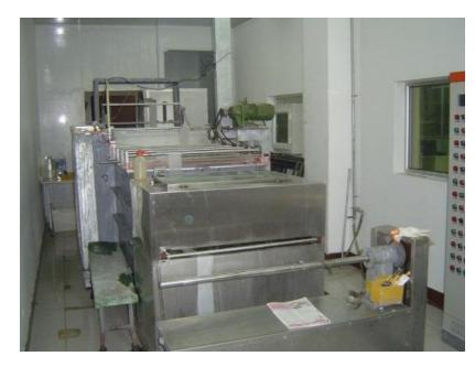
Figure 67: Film etching device at China Institute of Atomic Energy
