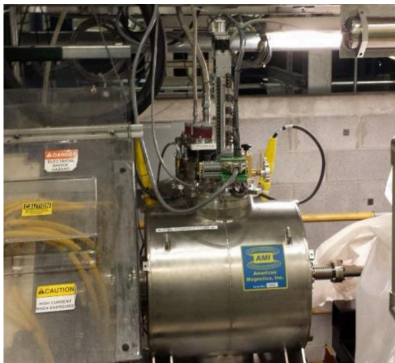
Figure 157: The Hall A Møller polarimeter target chamber installed on the beamline. The hardware above the cylindrical cryostat controls the vertical target ladder.
