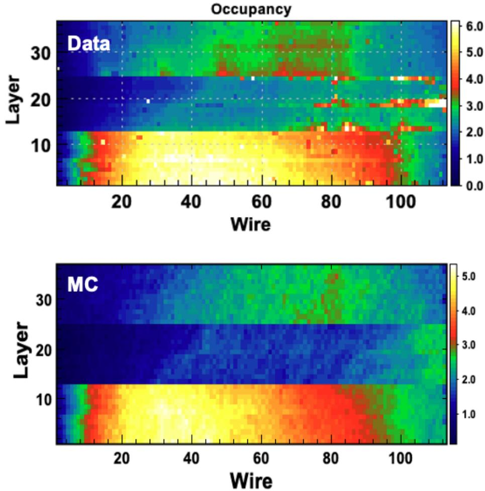
FIG. 26: DC occupancies as measured in CLAS12 and simulated in GEMC.
