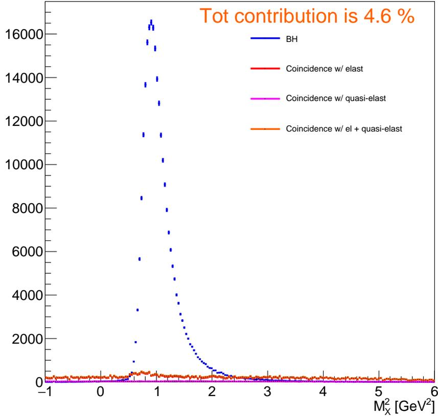
FIG. 41: Missing mass squared distribution electron-2MI P events for 200 days of running at  $10^{37}\text{cm}^{-2}\text{s}^{-1}$  luminosity. The blue distribution represents BH events, red represents the accidental coincidence of inclusive electrons and elastically produced muon pairs, pink is the coincidence with inelastic muon pairs, and orange is the sum of elastic and inelastic coincidences.
