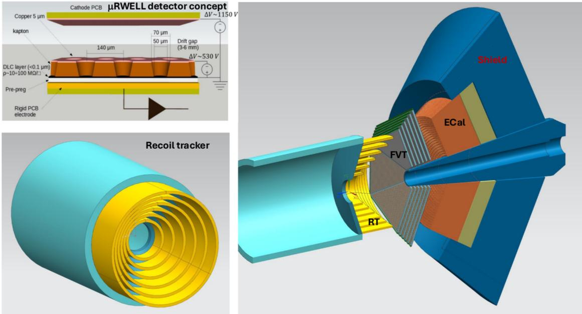
FIG. 25: On the left  $\mu$ RWELL MPGD concept (top) and the rendering of the barrel recoil detector (bottom). On the right, new detector elements of  $\mu$ CLAS12.
