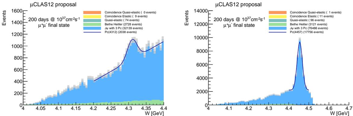
FIG. 56: Left: Hadronic mass  $W$  in the  $\mu$ CLAS12 acceptance, below 4.4 GeV. The invariant mass of the muon pair is restricted in the 2.7 to 3.2 GeV range. With the proposed integrated luminosity according to the model in [119], we expect to produce approximately 2000  $P_c(4312)$ .
