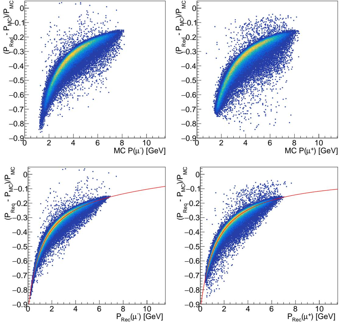
FIG. 37: Relative momentum loss ( $\Delta P/P$ ) as a function of generated momenta (top row) and reconstructed momenta (bottom row). correspond to negatively charged muons, while those on the right correspond to positively charged muons. The red curves in the bottom plots indicate the corresponding correction functions..
