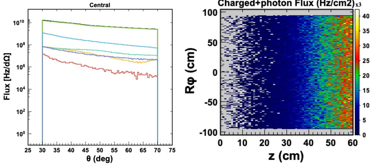
FIG. 32: Rates of particles at the cylindrical scoring plane located at 30 cm radius from the beam at the luminosity of  $10^{37} \text{ cm}^{-2} \text{ sec}^{-1}$ . Left: the rates for different particle types with 10 keV energy cut as a function of polar angle. Right: azimuthal and  $z$  distribution of rates of photons and charged particles.
