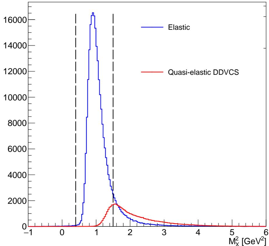
FIG. 39: Missing mass squared distribution for elastic (blue) and inelastic (red) muon pair production. Vertical dashed lines represent the missing mass cut.
