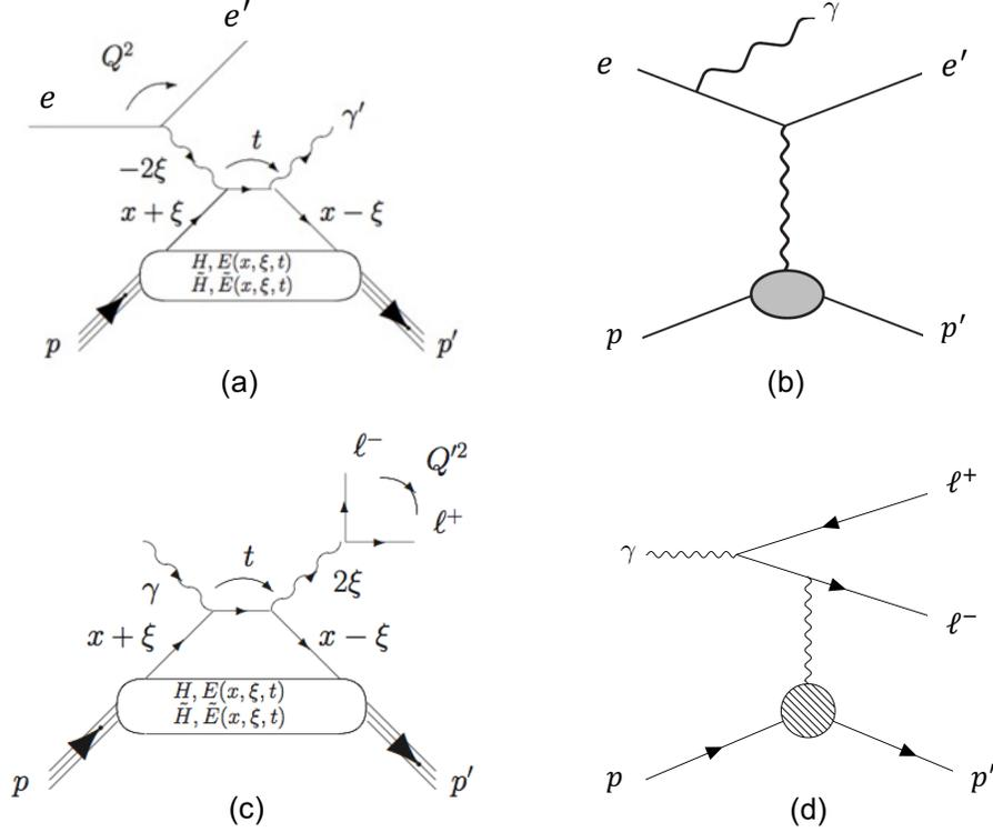
FIG. 2: Diagrams for Compton processes: (a) DVCS and (c) TCS processes, and accompanying Bethe-Heitler processes (b) and (d), respectively.
