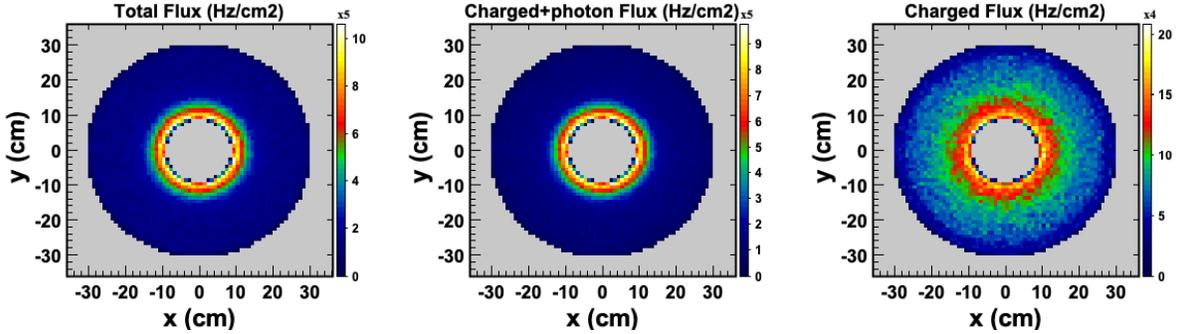
FIG. 31: Hit rates at the scoring plane before wECal at the luminosity of  $10^{37} \text{ cm}^{-2}\text{sec}^{-1}$ . Left: the rate for different particles as a function of polar angle with 15 MeV energy cut in the wECal. Right: the rate from charged particles with the same energy cut.
