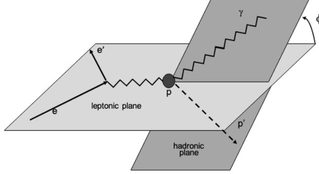
FIG. 3: Diagram of DVCS scattering planes. The angular harmonics of  $\phi$  between the leptonic and hadronic planes project out the interference term of the scattering amplitude.
