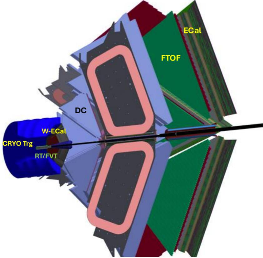
FIG. 28: GEANT4 rendering of the  $\mu$ CLAS12 detector,  $\mu$ GEMC.
