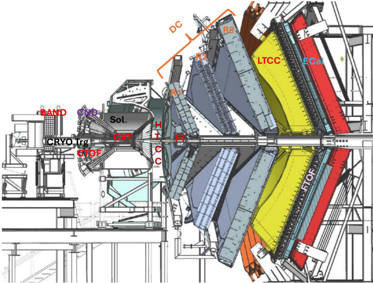
FIG. 20: The CLAS12 detector in Hall-B, mid-plane cut view. The detectors that will be removed/replaced are noted in red.
