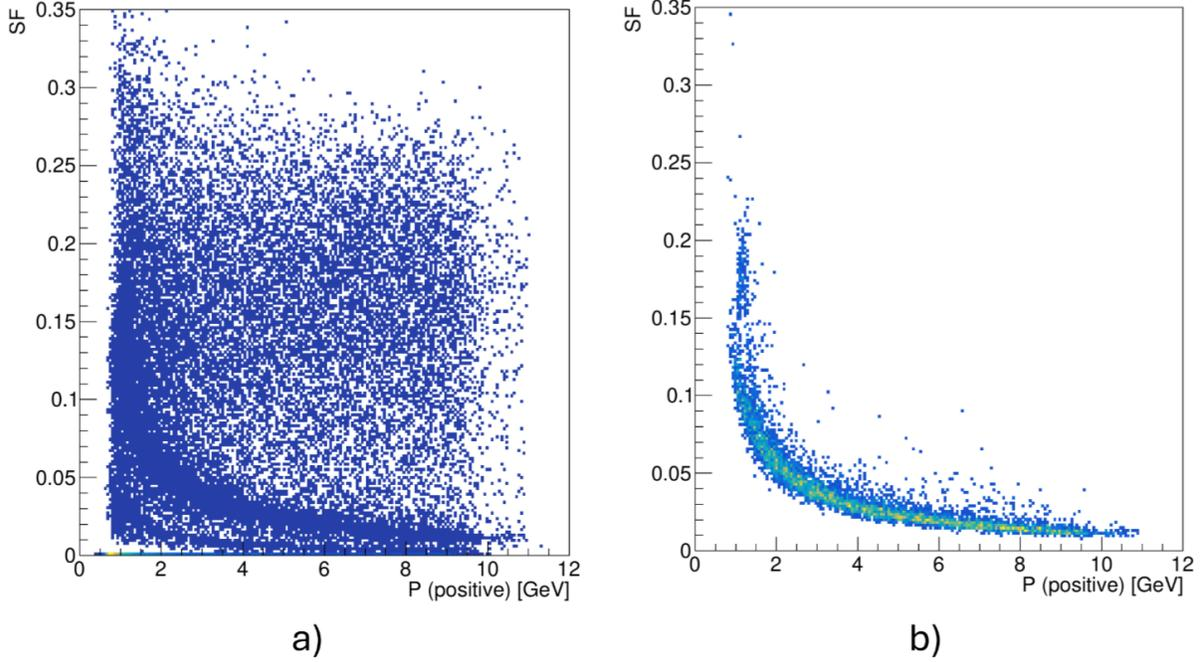
FIG. 34: A forward-ECal sampling fraction ( $SF = E_{cal}/p$ ) vs. momentum for  $\pi^+$ s that passed the calorimeter-shield and end up in fECal. Distribution in a) is for all pions, and b) those who survived a number of fECal strip cuts to select true MIP particles.
