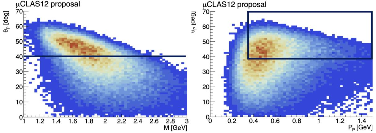
FIG. 57: Left: Proton polar angle as a function of the invariant mass of the muon pair. Right: Polar angle as a function of momentum for the proton. Events displayed are required to have a muon pair detected in  $\mu$ CLAS12. The black line shows the acceptance limit of the recoil detector. Events within this region are used to estimate the measurement yield.
