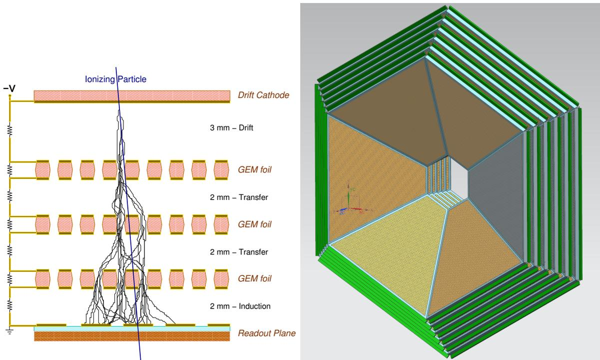
FIG. 24: On the left, the working principle of a triple GEM detector. On the right, rendering of a proposed 6-module GEM vertex tracker for  $\mu\text{CLAS12}$ .
