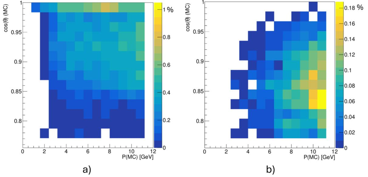
FIG. 35: A distribution of the fraction of positively (a) and negatively (b) charged MIP particles from simulated  $3\text{M } \pi^+$ s after cuts on the number strips in fECal. The original sample of pions was generated uniformly in momentum and  $\cos\theta$  using a GEANT particle gun.
