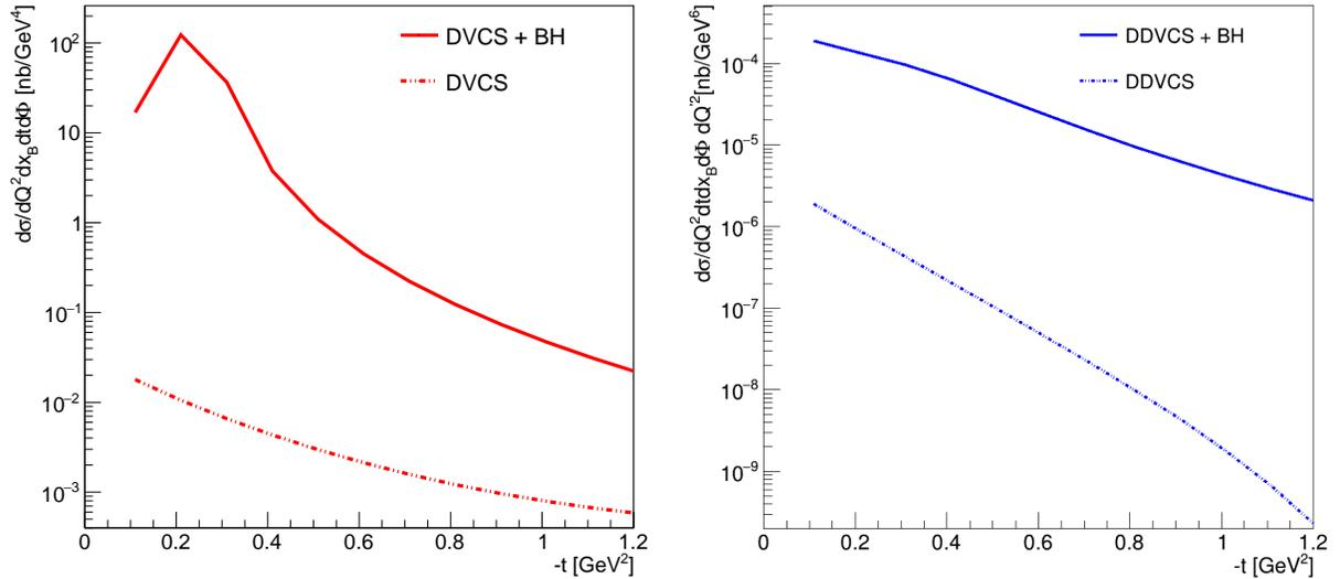
FIG. 13: Differential cross sections of DVCS (left) and DDVCS (right) processes with  $E = 10.6$  GeV electron beam. The scattered electron kinematics is fixed at  $Q^2 = 2.75 \text{ GeV}^2$  and  $x_B = 0.15$ .
