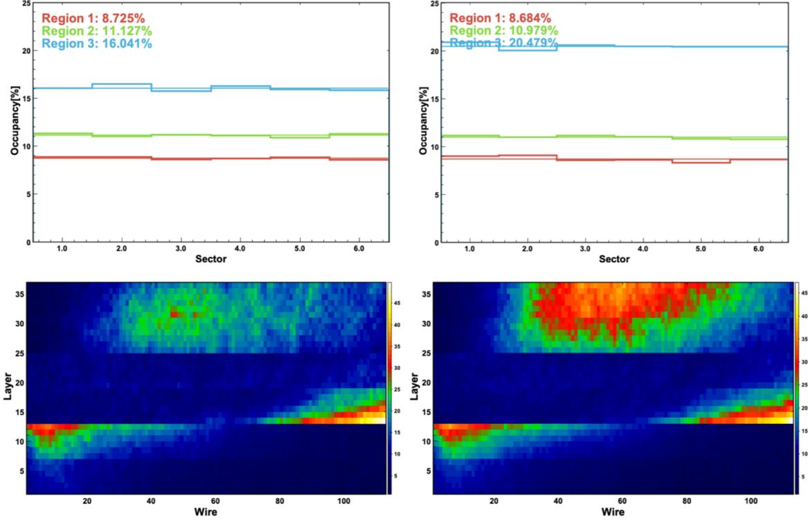
FIG. 29: The drift chamber occupancies at the luminosity of  $10^{37}\text{cm}^{-2}\text{s}^{-1}$  with a 30 cm thick lead shield downstream of the  $\text{PbWO}_4$  calorimeter. Left: occupancies with a 2 mm thick carbon shell on the back of the Region 3 DCs. Right: occupancies without the carbon shell. The top plots show the average occupancies per sector, and the bottom plots are occupancies as a function of the DC write number for three regions.
