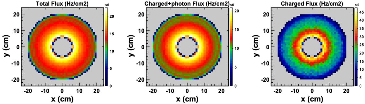
FIG. 30: Rates of particles with more than 10 keV energy at a luminosity of  $10^{37} \text{ cm}^{-2} \text{ sec}^{-1}$  crossing the scoring plane at 40 cm from the target center. Left: total rate; Middle: the rate charged particles and photons; and Right: the rate from charged particles only.
