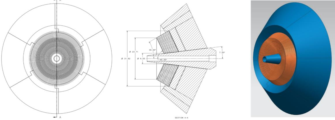
FIG. 23: The W-shield and PbWO<sub>4</sub> calorimeter.
