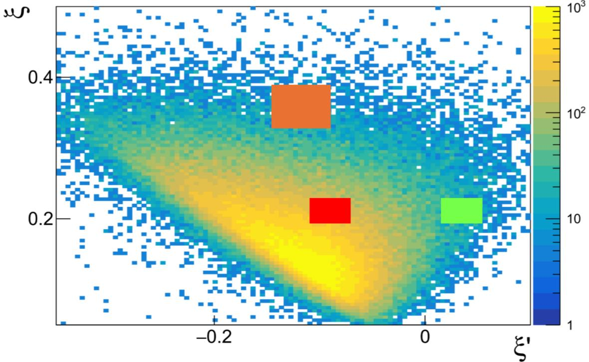
FIG. 45:  $\xi$  vs.  $\xi'$  distribution for reconstructed DDVCS+BH events. The boxes represent kinematic bins used to illustrate expected beam spin asymmetries in the time-like,  $Q'^2 > Q^2$ , and space-like,  $Q'^2 < Q^2$ , regions.
