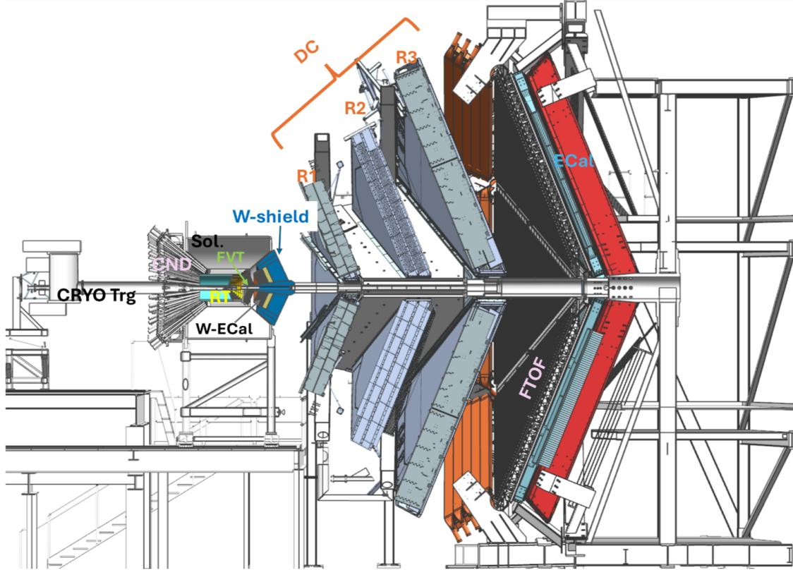
FIG. 22: The concept of the proposed DDVCS setup. The W-shield and  $\text{PbWO}_4$  calorimeter are installed in the place of HTCC. The FVT and the recoil tracker are inside the solenoid.
