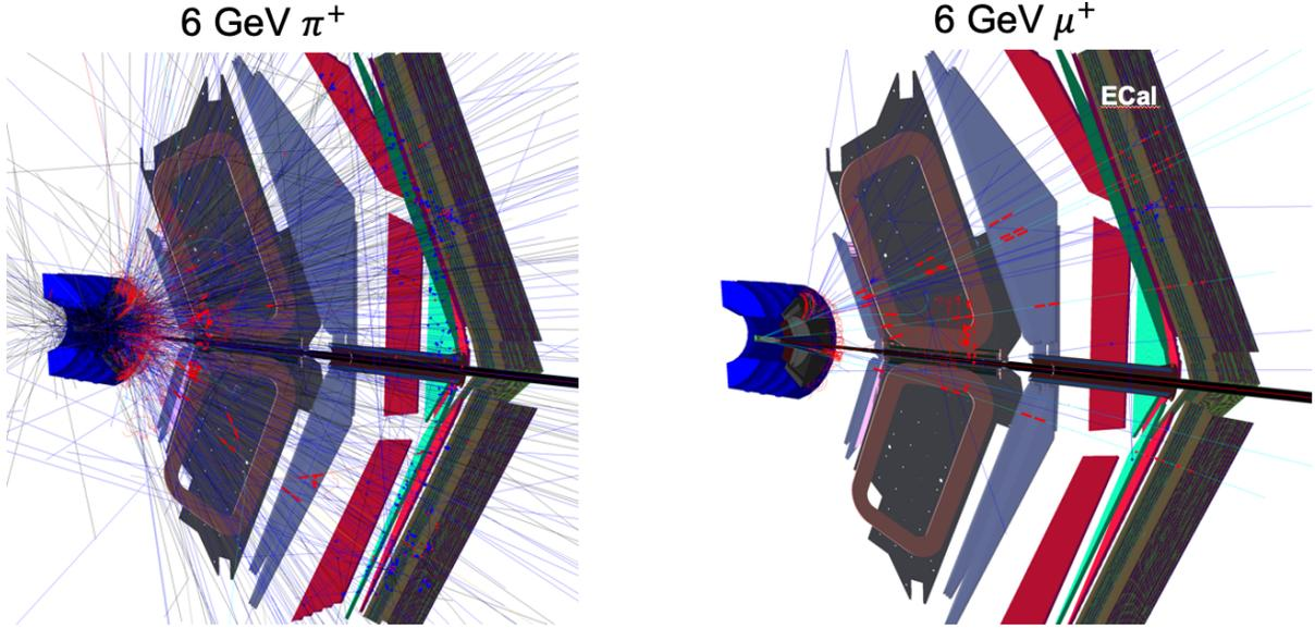
FIG. 33: Simulation of 6 GeV/c  $\pi^+$ s and  $\mu^+$  through the  $\mu$ CLAS12 GEANT4 model. Almost all pions interact in the wECal while muons punch through and get reconstructed in DC and fECal.
