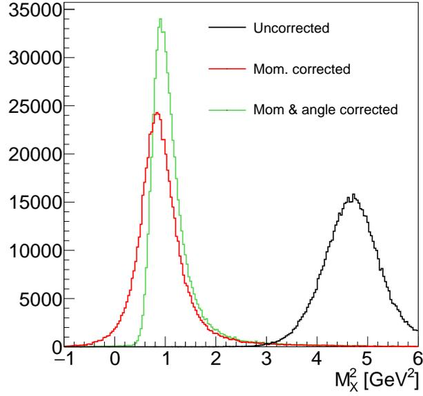
FIG. 38: The missing mass squared distribution of the reaction  $ep \rightarrow e' \mu^- \mu^+ X$ . The black distribution corresponds to the uncorrected data, the red distribution is obtained after applying momentum corrections to both muons, and the green distribution shows the result after additionally correcting the polar and azimuthal angles. .
