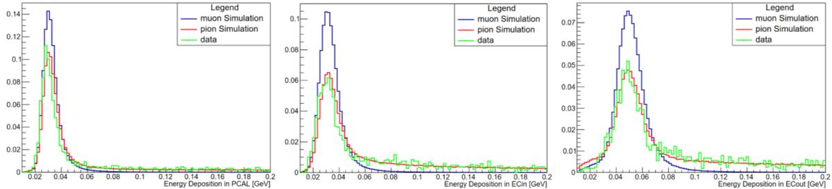
FIG. 27: The energy distribution for minimum ionizing particles ( $\pi^\pm$ ) in the fECal module, PCal, ECIn, and ECOOut. The green distributions are for data from RG-A, the red histograms are MC for  $\pi^\pm$ , and the blue histograms are for simulated  $\mu^\pm$ . The histograms are normalized to the total number of each sample.
