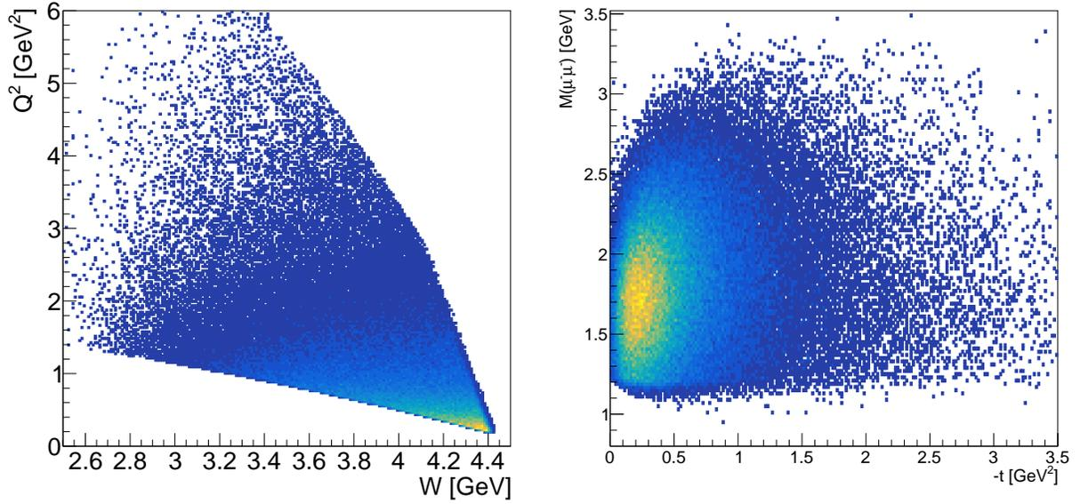
FIG. 43: Kinematic coverage of  $\mu$ CLAS12 for di-muon electroproduction with an 11 GeV electron beam. Left:  $Q^2$  vs.  $W = \sqrt{s}$  distribution, where limits are defined by detecting the scattered electron in the  $\mu$ CLAS12  $\text{PbWO}_4$  calorimeter. Right: Distribution of the invariant mass of lepton pairs detected in the  $\mu$ CLAS12 forward detector as a function of squared momentum transferred.
